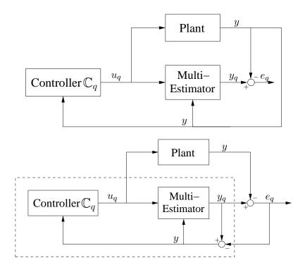
$\rightarrow$  The reason this transformation is useful is because, as we already discussed earlier, the control design should really be based on the design model (multi-estimator in the present setting) and not on the unknown plant itself.
