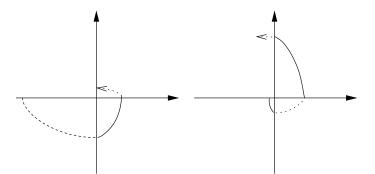
From this example, the instability mechanism is also quite clear: even though each system is stable, we catch it at the "peak" of its transient and switch to the other system, without giving it a chance to decay.
