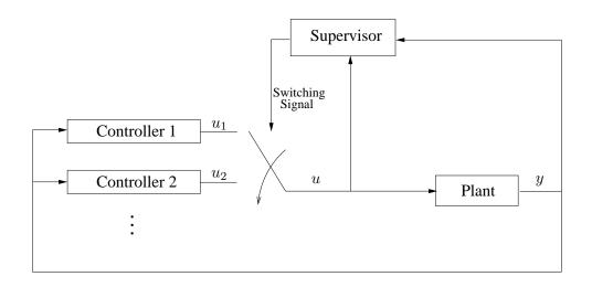
$\rightarrow$  The above figure suggests that the set of controllers is discrete (even finite). This is an option that was not possible in continuous adaptive control. However, we can still have a continuum of controllers and pick controllers from this continuous family one at a time.
