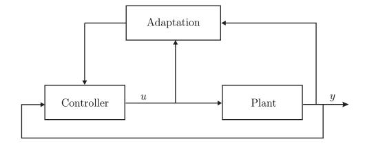
A priori, this is no different from any other (non-adaptive) dynamic feedback. But the main feature of the adaptive controller is that it achieves the control objective (regulation) despite *large-scale uncertainty* associated with  $\theta$  (which can be any real number). This is to be contrasted with *robust control* where uncertainty range is usually bounded and small.
