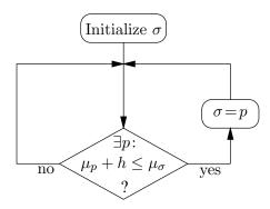
It remains to define the switching signal  $\sigma : [0, \infty) \to \mathcal{P}$ , which will give us the switching controller  $u(t) = -K_{\sigma(t)}x_{\sigma(t)}$ . One way to do this is by means of the so-called *hysteresis switching logic*, see figure.
