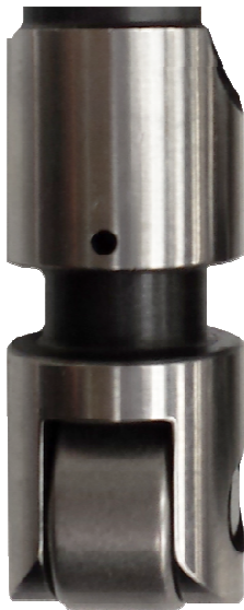
Figure 1: Stock un-modified solid roller lifters
