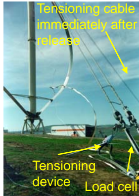
Tensioning device putting an impulse force load on the rotor (wide-band, transient deterministic)
