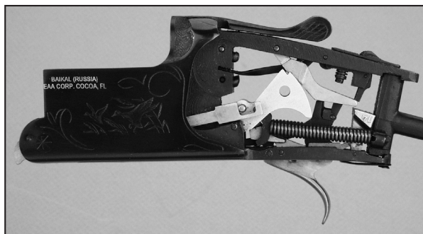
The trigger is mechanical, and pushing forward on the trigger blade from behind when the gun is cocked allows the shooter to switch barrel selection to the upper barrel first.
