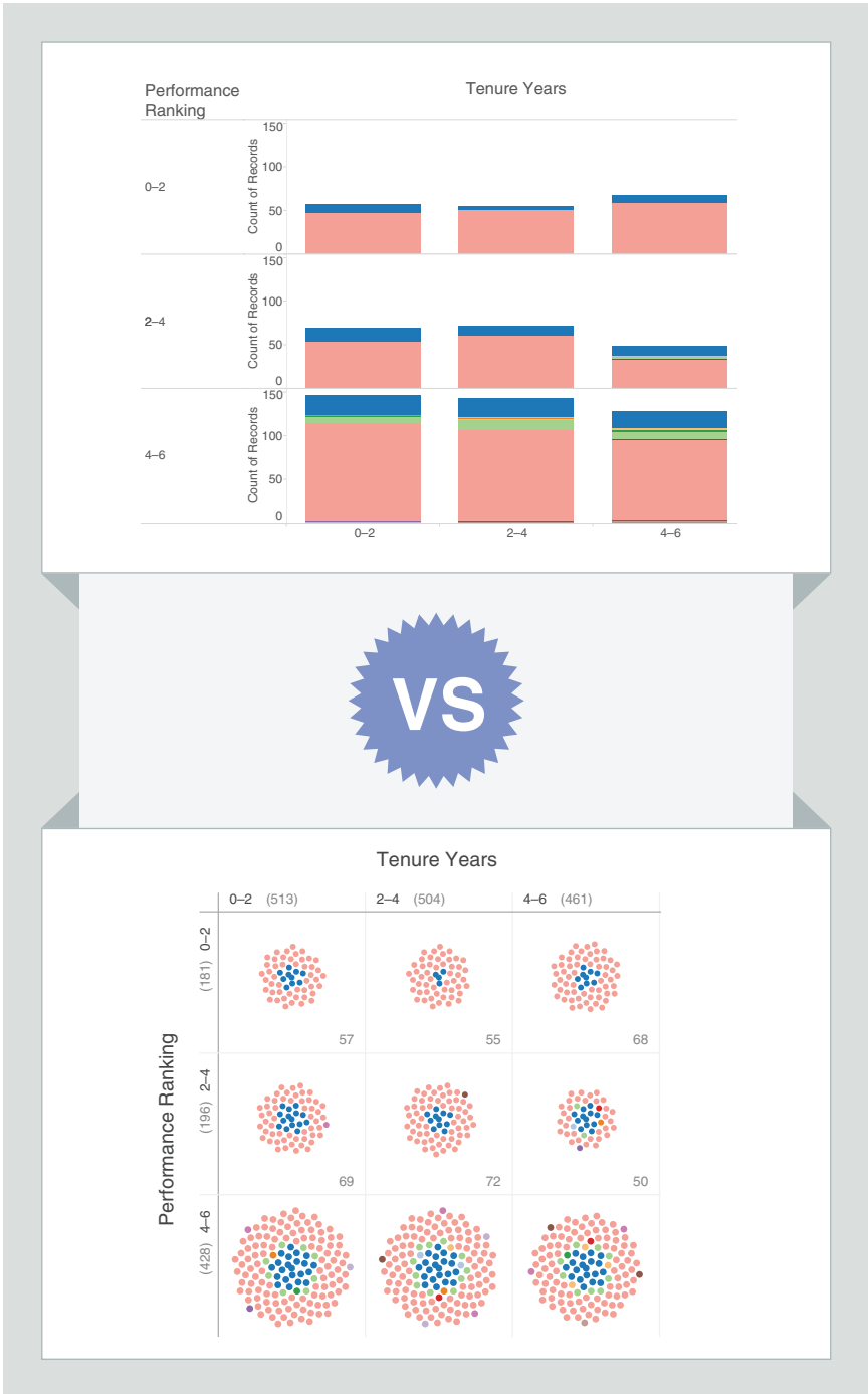
FIGURE 1.3.11 Stacked bar graph versus sunflower visualization: performance ranking versus tenure coloured by location
