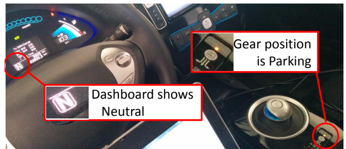
Figure 3: Changing the dashboard display of gear position.
