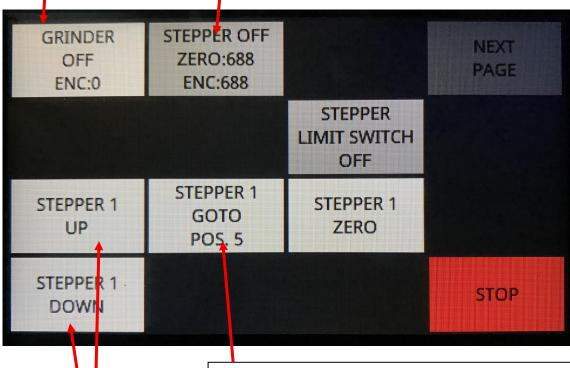
**STEPPER 1 GOTO POS. 5**: Stepper motor will move to ZERO position first and then to position 5. The final ENC value will be equal to ZERO value.
