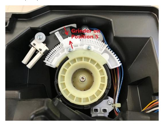
If the grinder is not in position 5 (i.e. the two markers are not aligned, see the right grinder on the above picture), the factory position can be restored by using the **STEPPER UP** or the **STEPPER DOWN** functions available in the load test mode.
