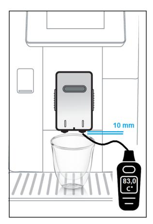
The optimal indicative temperature measurement for coffee should be 83°C±3°C.
