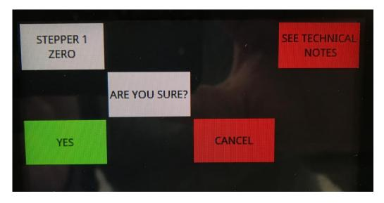
Press the YES button to confirm the execution of the ZERO STEPPER procedure.
