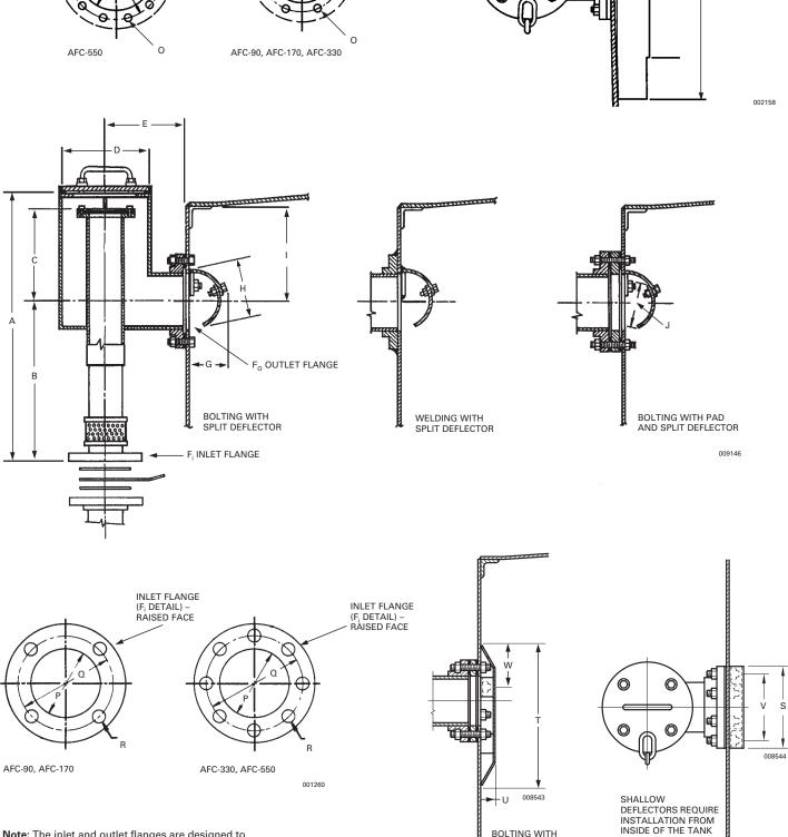
**Note:** The inlet and outlet flanges are designed to mate with ANSI 150 lb class flanges.
