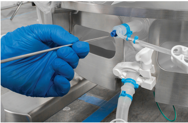
Figure 7. Temperature sample port.
