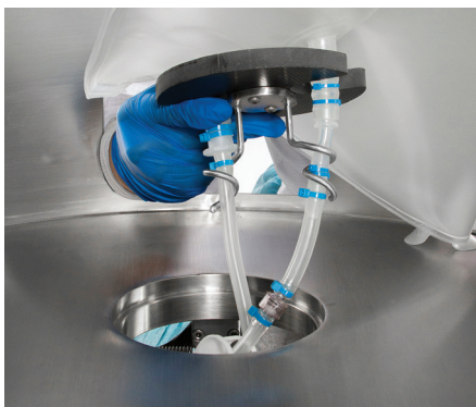
Figure 4. Sparge line support.
