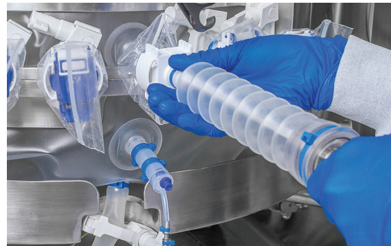
Figure 3. Bioreactor probe assembly.
