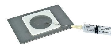
If the Patch is in a position which makes access to the Patch test chamber difficult, bend the Syringe needle as required.
