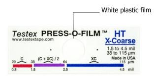
Remove the Testex Tape from the surface and place the replica between the anvils of the Testex Gauge, making sure that it is centred properly.
