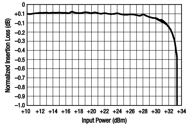
Figure 6. Normalized Insertion Loss vs Input Power
