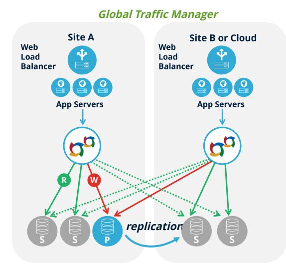
ScaleArc performs read/write split and geoload balance database traffic
