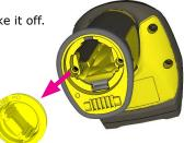
2. Hold the reader in an upright position and the battery will slide out of the handle. NOTE that you may need to shake the reader slightly.
