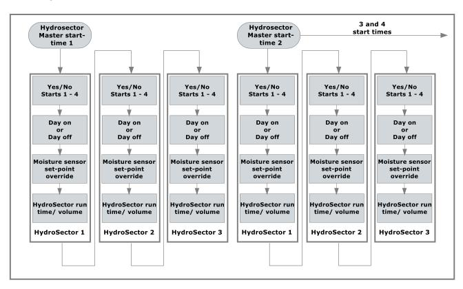
HydroSectors will run in sequence. If an override is triggered e.g. Moisture, day off, non acceptance of a master start time 1—4, the next H/sector in the sequence will start.
