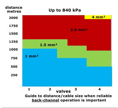
The chart shows the varying degree of performance in relationship to number of valves running, cable size, distance and operating pressure. The tests were performed using actual cable lengths and in workshop test conditions. High resistance and intermittent connections can effect the performance of the back-channel and valve actuation.
