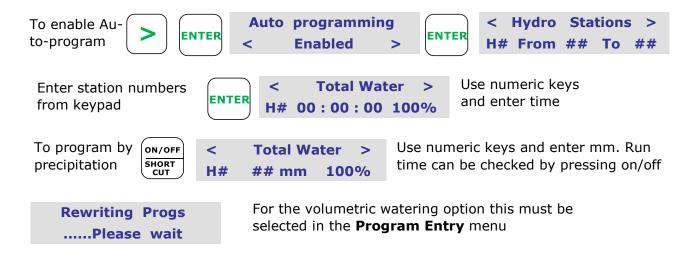
The HydroSectors are now selected. Stations have been allocated and watering times and/ or volumes have automatically been calculated for each valve/station and start times have been programmed.
