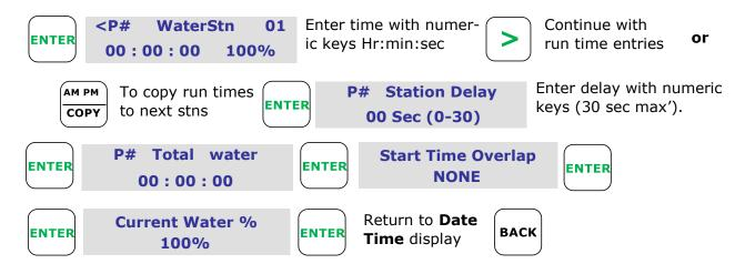
A basic program has now been entered using default factory option settings i.e. Time based station watering, no loop program, no auxiliary program and no station delays. The Master valve/pump start is at number 49.
