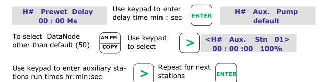
**Note.** The auxiliary pre-wet is the time the station runs without the dosing pump (auxiliary) running. The auxiliary run is the dosing pump run time. The balance of the time on the stations watering time is a post-wash time.
