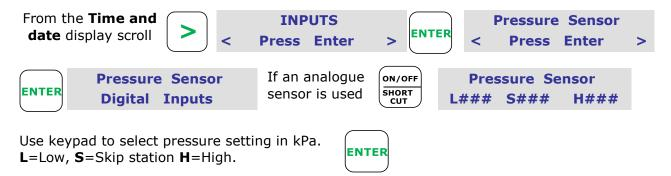
**Note.** If analogue sensor is not used - Pre-set sensors can be connected to the controller terminals [HP], [SP] and [LP]. (N/O contacts)
