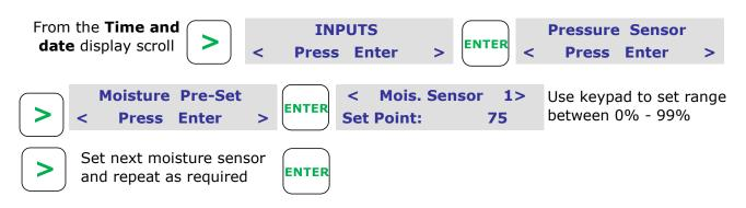
**Note.** The Moisture Pre-set is in Volumetric Water Content (ie a % of soil moisture). See moisture sensor guide which comes with sensors.
