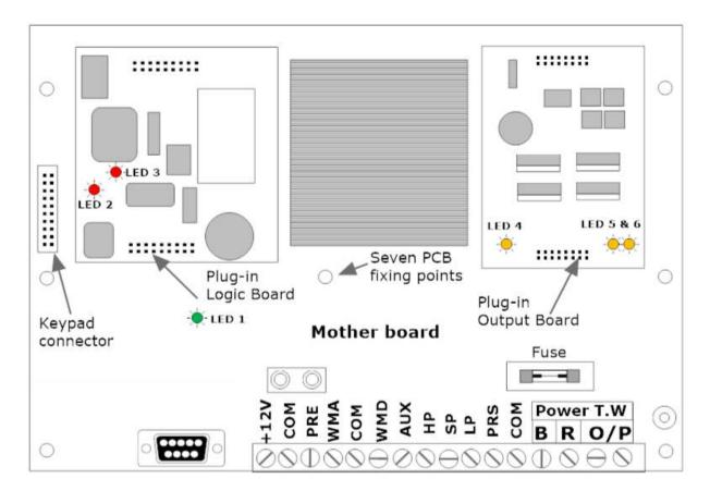
If it is suspected a fault is present at the controller and not in the field cabling or DataValves, proceed as follows:
