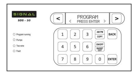
The key pad is a soft touch design with a audible beep to confirm contact. If a key is held down it will fast repeat. This is most helpful in the **Scroll** and **Back** keys.
