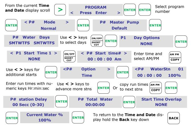
A basic program is now entered to run on a time basis. The pump/master valve number is 49 (default). No delays between stations have been set. No auxiliary/chemical injection program has been set to run. The program was not optioned for looping so it will start at the programmed times and finish at the end of the last station run time in a program. All default settings have been used.
