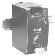
or extends the hold-up time after turn-off of the AC power. In times when the power supply provides sufficient voltages, the buffer module stores energy in integrated electrolytic capacitors. In case of mains voltage fault, this energy is released again in a regulated process. One buffer module can deliver 20A which can also be used to support peak current demands.
