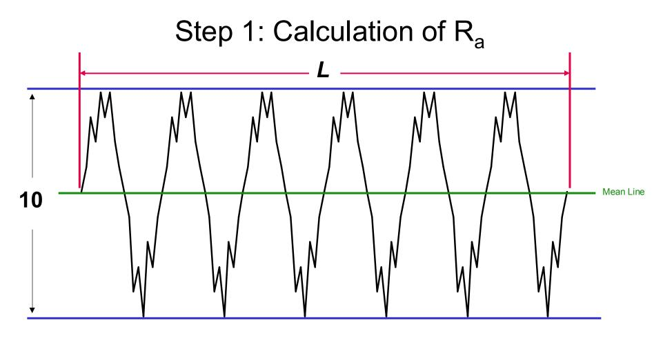
Filtered roughness profile with mean line, peak to valley is 10
