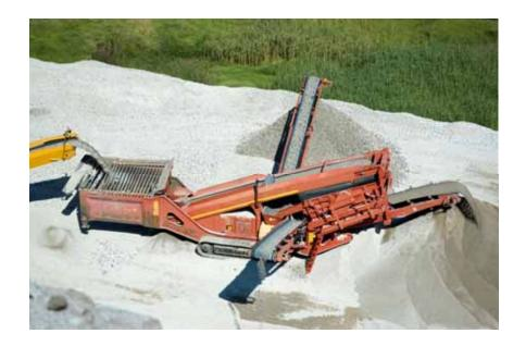
Cutoff functions in a method similar to this screening machine – sorting mixed material via screens, into size categories
