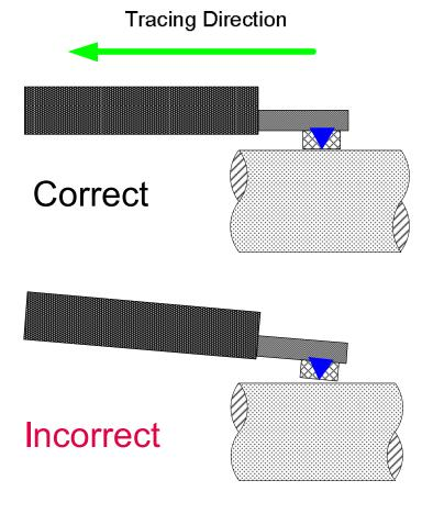
Skid or pickup parallel or level to the surface being measured
