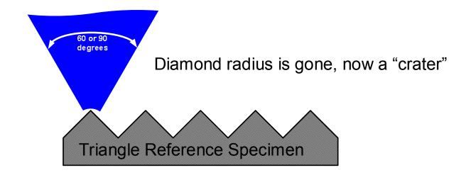
Trace of reference specimen indicates diamond is damaged
