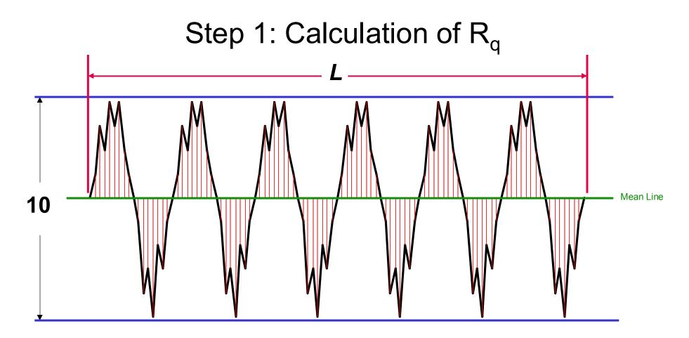
Filtered roughness profile with mean line, peak to valley is 10
