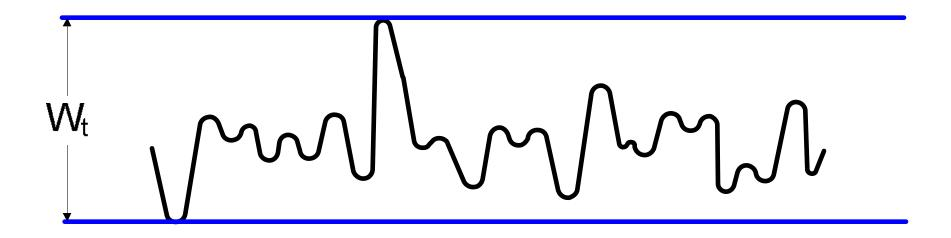
Generally, a maximum peak-to-valley measurement of waviness (roughness has been filtered out)
