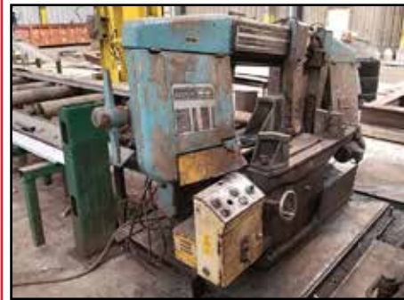
DAITO ST4565 Horizontal Band Saw w/32' x 52" Power Feed & 25' Steel Roll Power Conveyors
