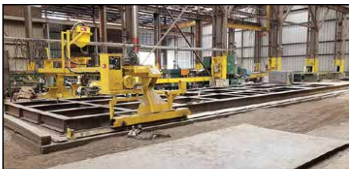
Sub-Arc Track Seam Welder, 189" x 52' Table w/Mighty-Mac HD Vacuum System
