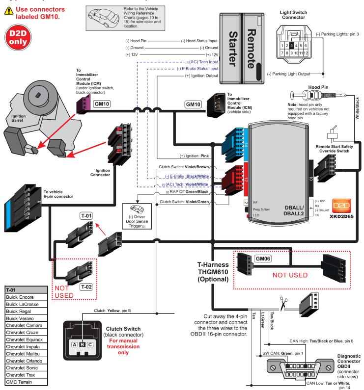
[1] Tach wire is an optional connection required on some remote starters, which do not support a tach signal in D2D.
