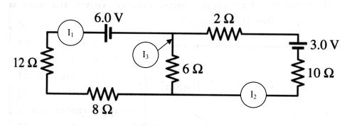
$[I_1 = 0.292 \text{ A}, I_2 = 0.264 \text{ A}, I_3 = 0.0278 \text{ A}]$
