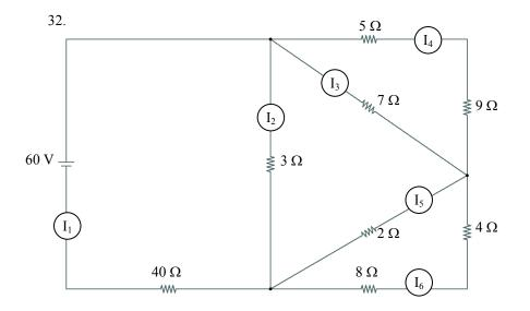
$[I_1\!\!=\!\!1.43 \text{ A } I_2\!\!=\!\!0.97 \text{ A } I_3\!\!=\!\!0.305 \text{ A } I_4\!\!=\!\!0.153 \text{ A } I_5\!\!=\!\!0.39 \text{ A } I_6\!\!=\!\!0.067 \text{ A}]$
