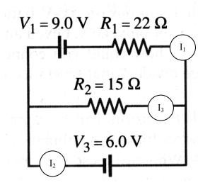
$[I_1 = 0.681 \text{ A}, I_2 = 1.08 \text{ A}, I_3 = 0.40 \text{ A}]$
