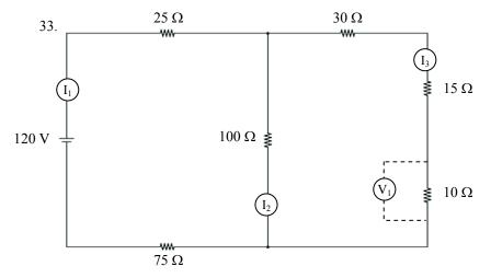
$[I_1 = 0.886 \text{ A } I_2 = 0.314 \text{ A } I_3 = 0.571 \text{ A } V_1 = 5.71 \text{ V}]$
