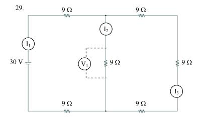
$[I_1=1.21 \text{ A } I_2=0.91 \text{ A } I_3=0.30 \text{ A } V_1=8.17 \text{ V}]$
