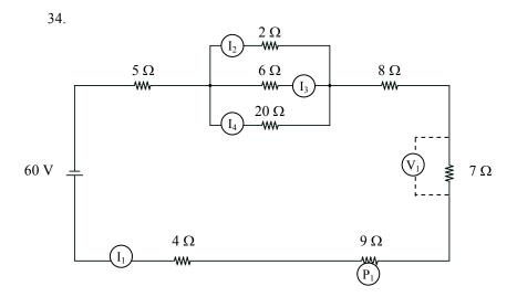
$[I_1 = 1.74 \text{ A } I_2 = 1.22 \text{ A } I_3 = 0.406 \text{ A } I_4 = 0.122 \text{ A } V_1 = 12.2 \text{ V } P_1 = 27.4 \text{ W}]$
