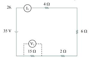
$[I_1 = 1.3 \text{ A V}_1 = 19.4 \text{ V}]$
