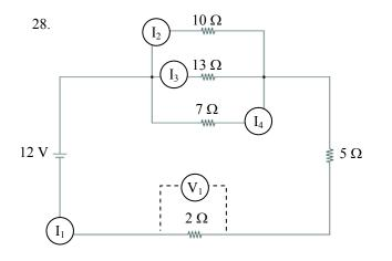
$[I_1=1.18 \text{ A } I_2=0.37 \text{ A } I_3=0.29 \text{ A } I_4=0.53 \text{ A } V_1=2.36 \text{ V}]$
