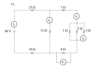
$[I_1=2.1 \text{ A } I_2=1.1 \text{ A } I_3=1.0 \text{ A } I_4=0.18 \text{ A } V_1=9 \text{ V}]$
