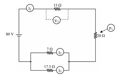
I<sub>1</sub>=2 A, I<sub>2</sub>=1.43 A, I<sub>3</sub>=0.57 A, V<sub>1</sub>=30V, P<sub>1</sub>=80 W
