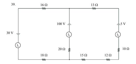
$[I_1 = 2.13 \text{ A } I_2 = 0.749 \text{ A } I_3 = 2.88 \text{ A}]$
