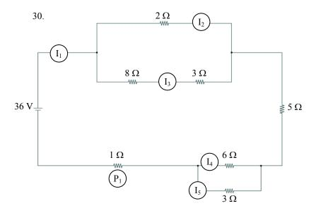
[I<sub>1</sub>=3.71 A I<sub>2</sub>=3.14 A I<sub>3</sub>=0.571 A I<sub>4</sub>=1.24 A I<sub>5</sub>=2.47 A P<sub>1</sub>= 13.8 W]
