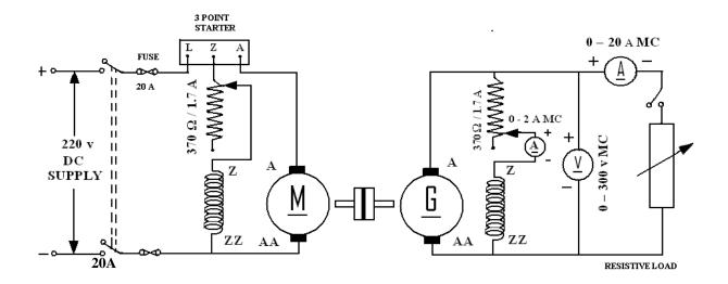
Fig - 2.1 DC Shunt Motor - Shunt Generator Set
