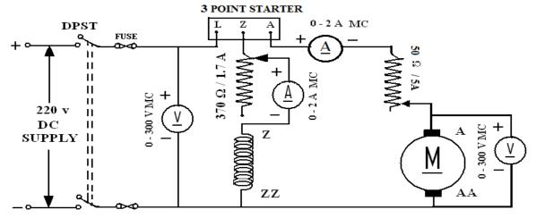
Fig – 11.1 DC Shunt Motor
