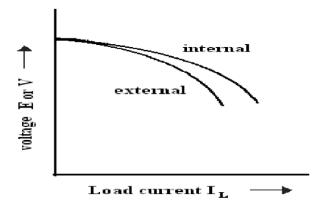
Fig - 2.2 Internal and External Characteristics of DC Shunt Generator
