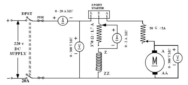
Fig – 7.1 DC Shunt Motor
