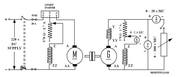
Fig - 4.1 DC Shunt Motor - Compound Generator Set
