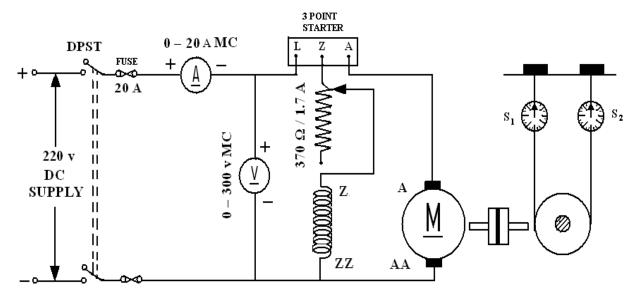
Fig – 9.1 DC Shunt Motor with Brake Drum
