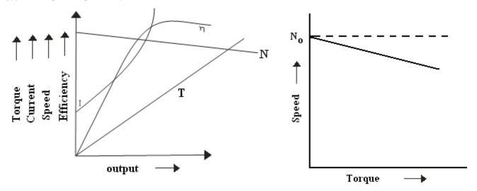
Fig – 8.2 Performance Characteristics of Compound Motor
