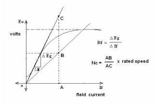
Fig - 1.2 Magnetization Characteristics Curve
