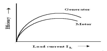
Fig – 7.2 Load Characteristics of DC Shunt Motor and Generator
