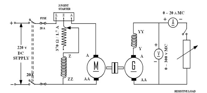
Fig - 3.1 DC Shunt Motor - Series Generator Set
