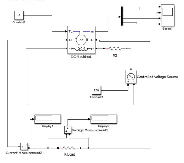
Fig - 13.1Circuit Diagram of Open Circuit Characteristics of Dc Shunt Generator
