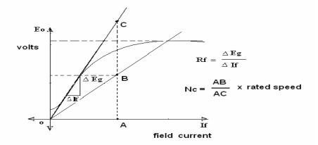
Fig - 12.2 Magnetization Characteristics Curve
