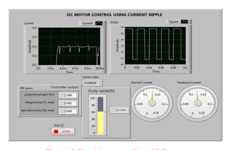
Fig - 14.2 Closed loop controlling of DC motor
