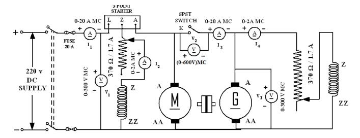
Fig - 5.1 Identical DC Shunt Machines
