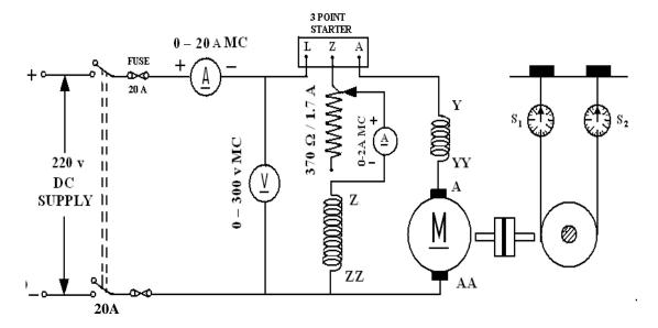
Fig – 8.1 DC Compound Motor with Brake Drum
