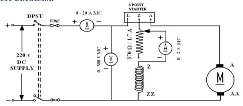
Fig – 7.1 DC Shunt Motor
