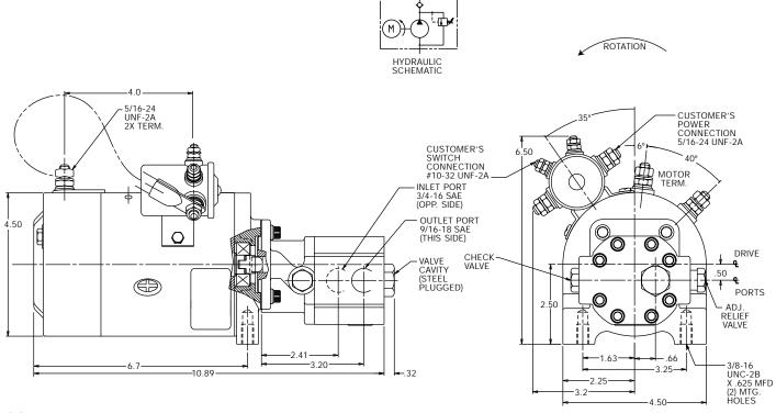
Motor: 12 Volt DC, 2 Terminal, Wound Field, Light Duty, 3" Motor, No Start Switch,
