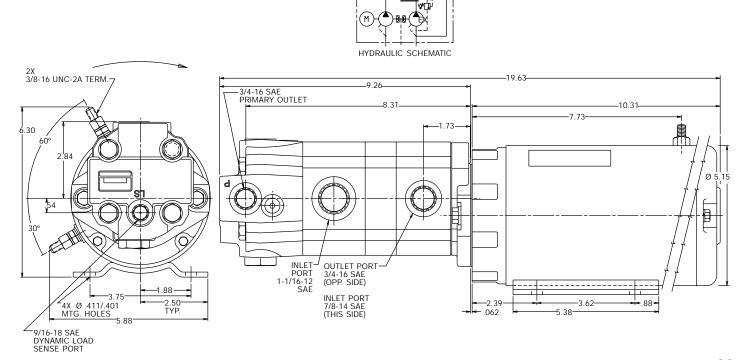
Motor: 24 Volt DC, 2 Terminal, Wound Field, Extended Duty, Sealed Motor, Heavy Duty 4 Terminal Start Switch with Boots, Motor Foot Mounting
