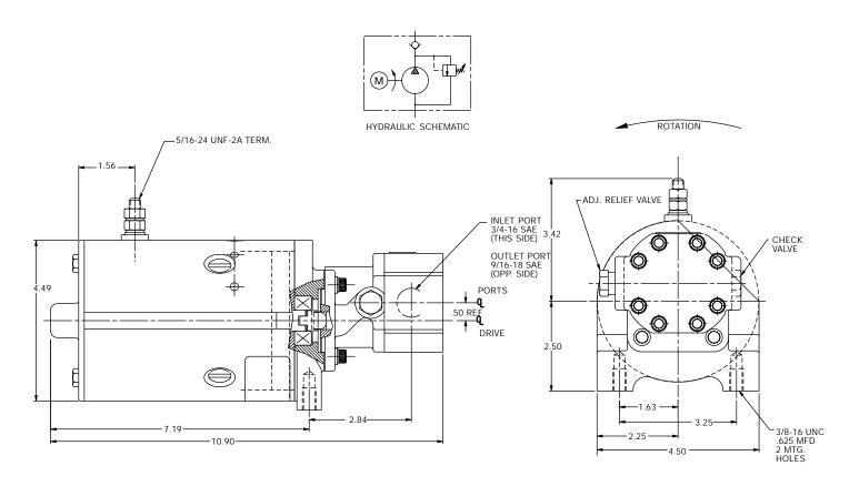
Motor: 12 Volt DC, 1 Terminal, Wound Field, Low Duty, Standard 4.5" Motor, 3 Terminal Start Switch with Boots, and "Horseshoe" Mounting
