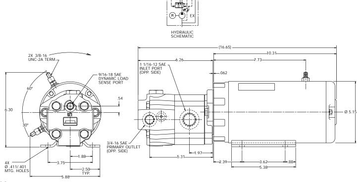
Motor: 24 Volt DC, 2 Terminal, Wound Field, Extended Duty, Sealed Motor, No Start Switch, Motor Foot Mounting
