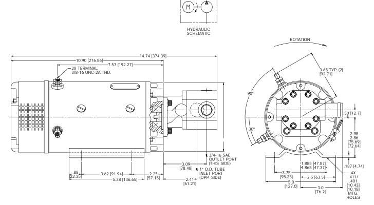
Motor: 12 Volt DC, 2 Terminal, Wound Field, Extended Duty, 5" Motor, UL Approved,
