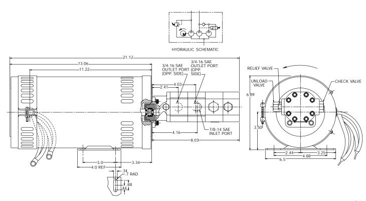
Pump: GC Series Pump, Two Section, No Valves, Flex Coupling Drive for Low Noise Operation
