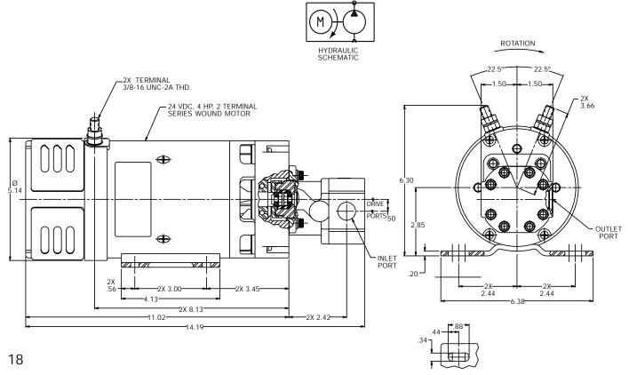
Pump: GC Series Pump, Two Section, No Valves, Flex Coupling Drive for Low Noise Operation
