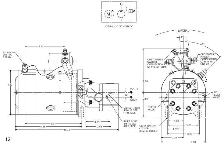
Motor: 12 Volt DC, 2 Terminal, Wound Field, Medium Duty, Standard 4.5" Motor, UL Approved, 4 Terminal Start Switch with No Boots, and Motor Foot Mounting
