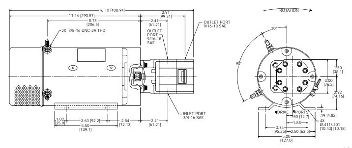
Motor: 48 Volt DC, 2 Terminal, Permanent Magnet, Extended Duty, Thermal Overload Protection, Motor Foot Mounting
