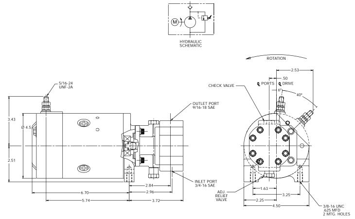
Motor: 12 Volt DC, 2 Terminal, Wound Field, Medium Duty, Standard 4.5" Motor, UL Approved, 4 Terminal Start Switch with No Boots, and "Horseshoe" Mounting
