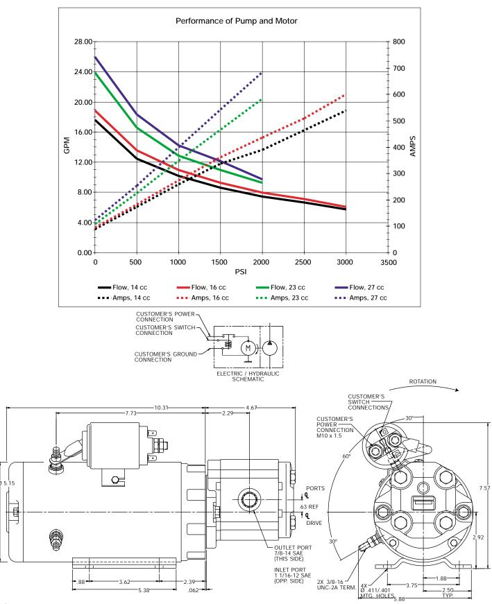
Motor: 24 Volt DC, 2 Terminal, Wound Field, Extended Duty, Sealed Motor, Heavy Duty 4 Terminal Start Switch with Boots, Motor Foot Mounting
