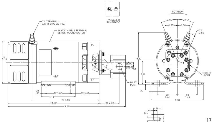
Pump: GC Series Pump, Single Section, No Valves, Flex Coupling Drive for Low Noise Operation
