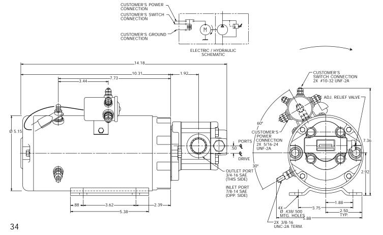
Motor: 24 Volt DC, 2 Terminal, Wound Field, Extended Duty, Sealed Motor, No Start Switch, Motor Foot Mounting
