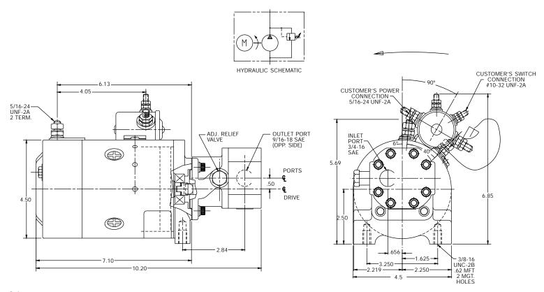
Motor: 24 Volt DC, 2 Terminal, Wound Field, Medium Duty, Standard 4.5" Motor, UL Approved, 4 Terminal Start Switch with Boots, Motor Foot Mounting with Weld Nuts
