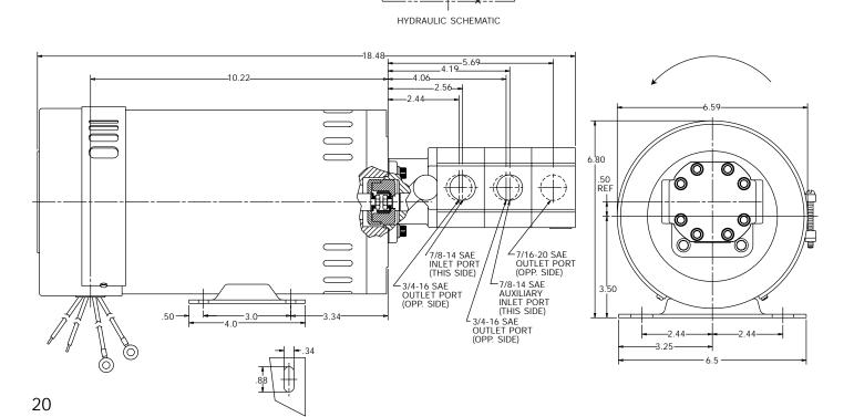
Motor: 24 Volt DC, 2 Terminal, Permanent Magnet, Extended Duty, Open Drip Proof, No Start Switch, Motor Foot Mounting
