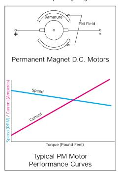
Permanent magnet motors generally run at a nominal speed of 1800 RPM (although other speeds are available). These motors have a lower stall torque than wound field motors, but are more efficient and exhibit superior thermal characteristics which make them more suitable for continuous duty applications. Some of the most common applications of permanent magnet motors are power steering and fuel systems.
