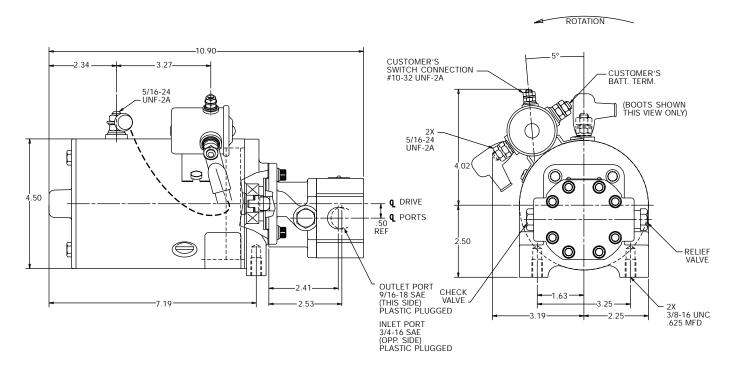
Motor: 12 Volt DC, 2 Terminal, Wound Field, Medium Duty, Standard 4.5" Motor, UL Approved, No Start Switch, with "Horseshoe" Mounting
