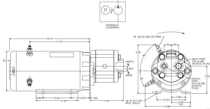
Motor: 24 Volt DC, 2 Terminal, Wound Field, Extended Duty, Sealed Motor, Heavy Duty 4 Terminal Start Switch Without Boots, Motor Foot Mounting
