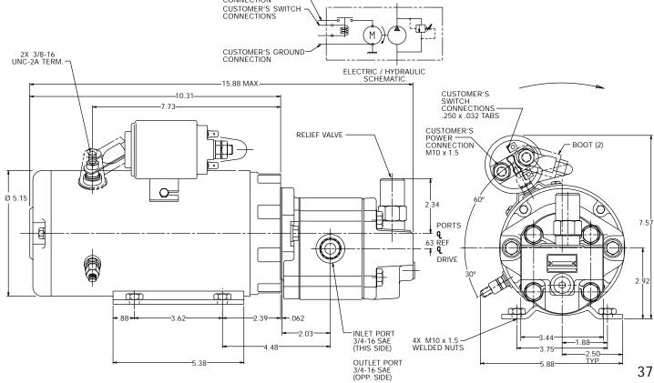
Motor: 24 Volt DC, 2 Terminal, Wound Field, Extended Duty, Sealed Motor,
