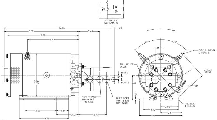
Pump: PB Series Pump, Single Section, Check Valve, Relief Valve, Solenoid Release Valve with Manual Override (L-H-L), Tang Drive
