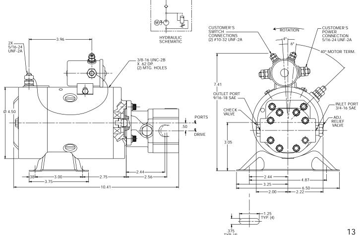
Motor: 24 Volt DC, 2 Terminal, Wound Field, Medium Duty, Standard 4.5" Motor, UL Approved, 4 Terminal Start Switch with No Boots, and "Horseshoe" Mounting.
