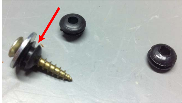
figure 42: additional grommet on the screw
