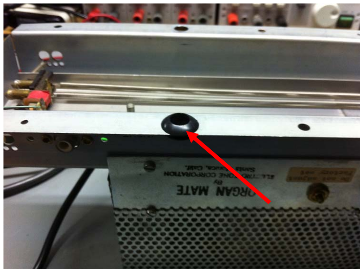
figure 41: spring unit stuffed with a new rubber grommet
