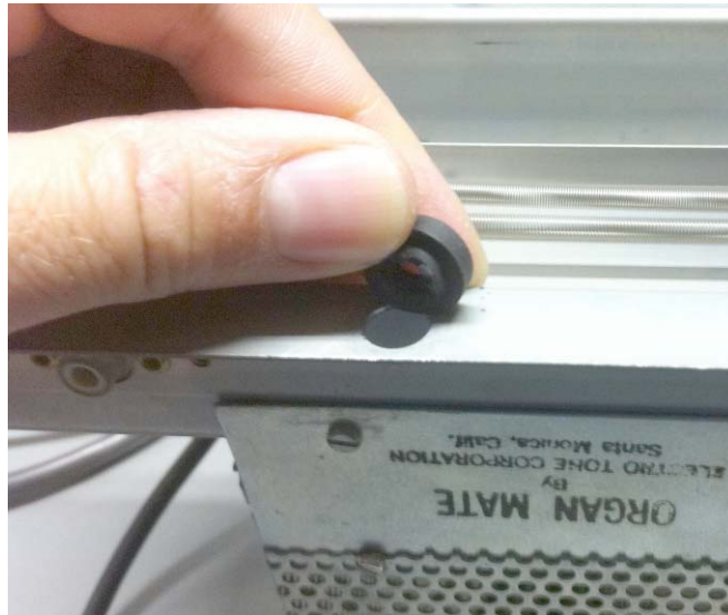
figure 38: old rubber grommets- falling into pieces when trying to remove
