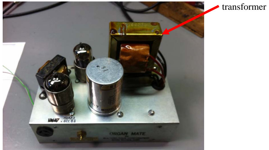
figure 30: transformer turned by 90°
