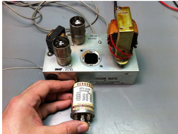
figure 25: multisection capacitor removed
