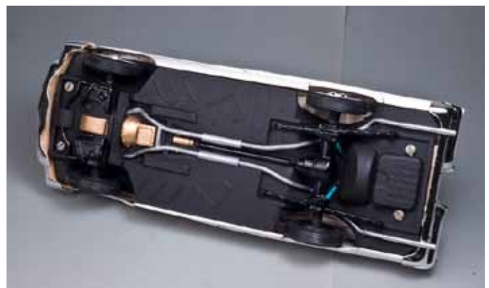
The original one-piece chassis was detail-painted to look somewhat more realistic. Some styrene tubing represents glass-pack mufflers under the center of the car. The stock mufflers and tailpipes were replaced with polished aluminum tube. Unpainted areas visible inside the body and bumpers would be painted flat black before final assembly. More photos on following page...
