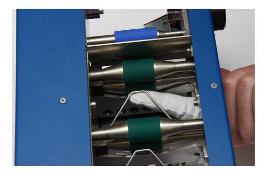
7. After cleaning leave the machine to dry. Slide the Top Cover back (please note that the Top Cover is not symmetrical so needs to be put back in the right direction). The machine is now ready to go.
