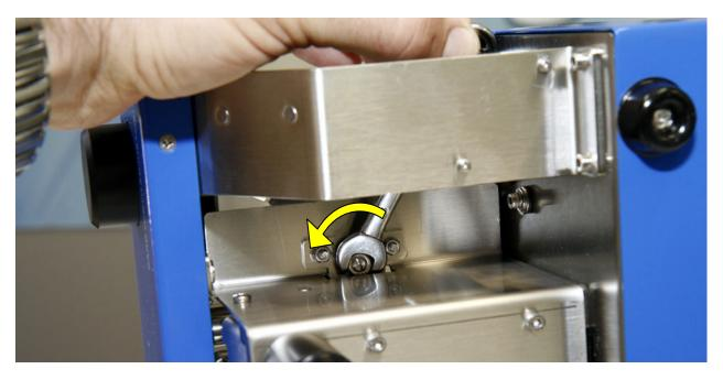
3. Put the Feeler gauge blade with the desired thickness into the Feeder Gap. If the blade does not fit (Feeder Gap is too small) rotate card support mushroom anticlockwise (when looking from the bottom) using a small flat screwdriver. This makes the gap bigger and will allow the Feeler Gauge blade to fit. Some early models (serial numbers from 4001 – 4012) are fitted with a card mushroom without a screwdriver slot. In this case the mushroom has to be rotated by hand.
