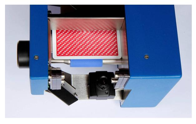
3. Rotate the Bottom Mushroom Knob clockwise until the mushroom touches the card in such a way that the card cannot be moved by hand. Do not over tighten. Then rotate the Knob a 1/4 turn counterclockwise. Use flat part of the knob to define a 1/4 turn:
