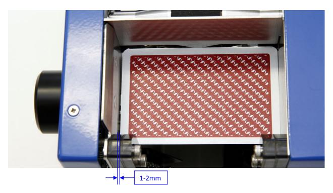
It may be necessary to adjust the Feeder width every time a new type (size) of card is used.
