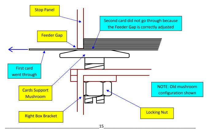
The correct Feeder Gap size is essential for proper Dealer4 operation. If the gap is too small it will be difficult or impossible to fit the cards through the gap. If the gap is too large two cards can through at the same time or the second card can block the first card.
