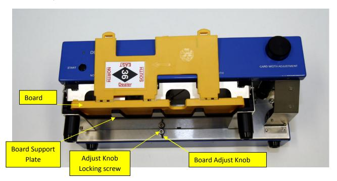
To adjust the Board Pocket, a 3.0mm Alan key is required. The Board Pocket adjustment is performed by rotating the Board Adjust Knob located under the Board Support Plate:
