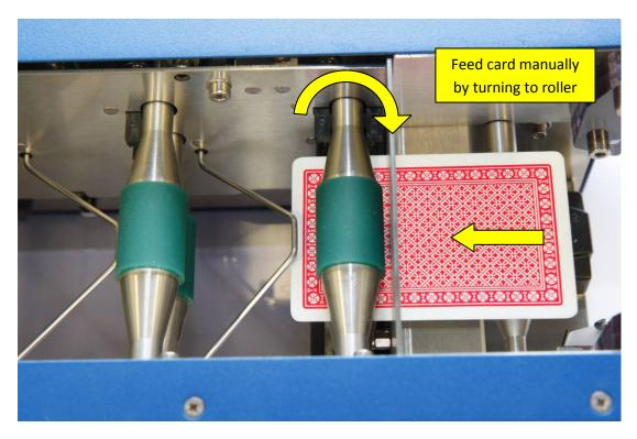
Insert card manually, and check the clearance between the gate and the card. In the lower position the gate should be around 1mm below the card. In the raised position the gate should be around 2mm above the card.
