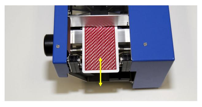
2. While the first card is still in the Feeder Gap try to fit a second one into the gap. This should be not possible. If the second card can fit into the gap even only slightly it means that gap is too large.
