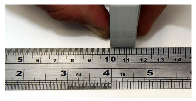
If card thickness is known the correct gap size can be calculated by multiply card thickness by 1.2 to 1.4.
