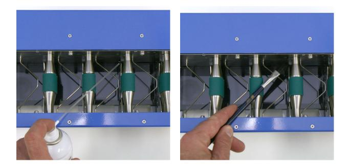
The best access to clean the first photointerruptor is from the Feeder side:
