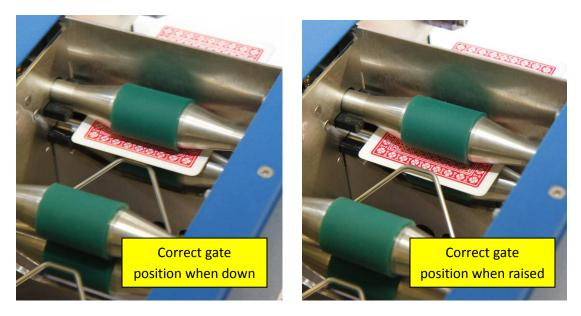
4. Once a problem gate has been identified, disconnect the machine completely and gently bend the gate as required.
