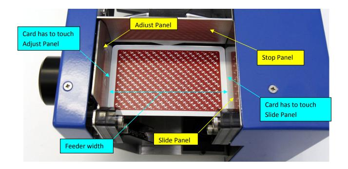
Then rotate adjustment knob 1.5 turns clockwise. This will move adjust panel by around 1.6mm and provides the correct Feeder width:
