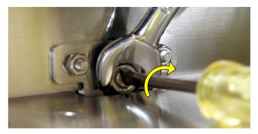
5. Using the 8mm spanner to lock the locking nut:
