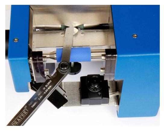
3. With the Feeler Gauge blade in this position rotate bottom mushroom knob clockwise until it touches the blade. Do not use to much force in this step – if the mushroom is rotated too much the Feeler Gauge blade may become difficult to remove. The Feeler Gauge should be tight in the gap but possible to remove without too much force.
