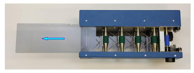
1. Take out the Machine cover by sliding it out to the left as shown:
