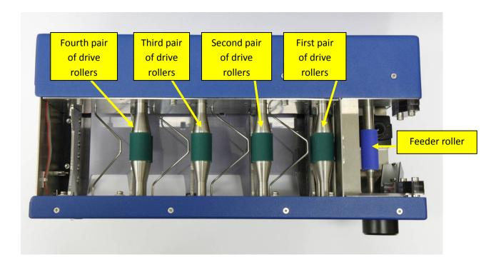
Typically the first pair of rollers is worn the quickest because every card goes through this pair. The machine can still be used in this condition but the dealing process will become slow to the point where dealing will become impossible. It is therefore recommended that when roller wear is discovered – the machine should be sent in for a service.
