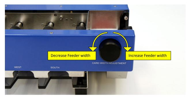
To adjust the card width, put one card into the Feeder and by turning adjustment knob set the adjust plate to touch the card on side:
