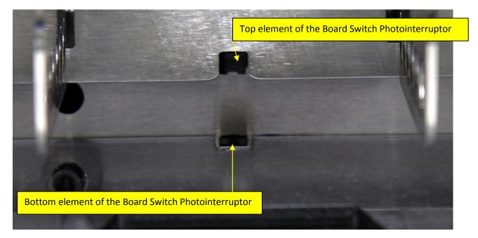
If any of the photointerruptors are too dirty the light beam can be blocked and Dealer4 will not operate correctly.
