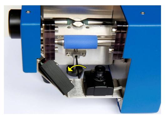
2. Insert the 0.4mm Feeler Gauge blade into the feeder gap.
