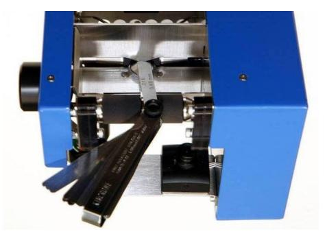
4. With Feeler Gauge blade in the position shown above, rotate the mushroom clockwise until it touches the blade. Do not use to much force in this step – if the mushroom is rotated too much the Feeler Gauge blade may become difficult to remove. The Locking nut should be held by a spanner during this step to not disturb the rotation of the mushroom
