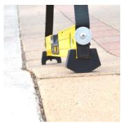
a wider stance to reduce the possibility of tipping and imbalances. The SmartTool™ offers objective and detailed slope measurements in degrees, percent slope, and pitch to 0.1 degree of resolution and accuracy. Using a standard 9-volt battery.
