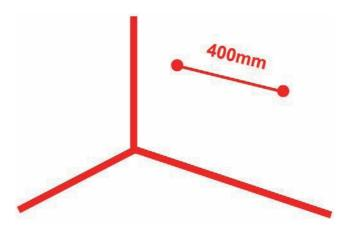
To mount the Sound Bar you need to have 400 mm of horizontal space on the wall.
