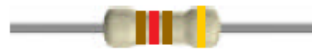
Figure G1 Image of a 120 Ohm resistor. Brown, Red, Brown with +/- 5% tolerance (Gold)
