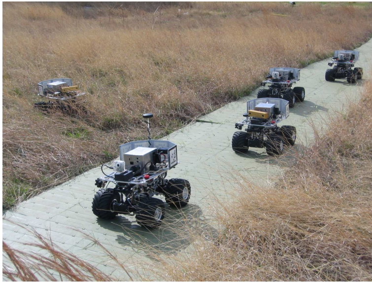
Figure 22: The convoy proceeds. The lead robot travels autonomously through the preassigned waypoints. Using communication, the other robots follow the leader in a line. Each follower attempts to drive at a safe distance from its preassigned leader. The robots safely traverse the path in formation.
