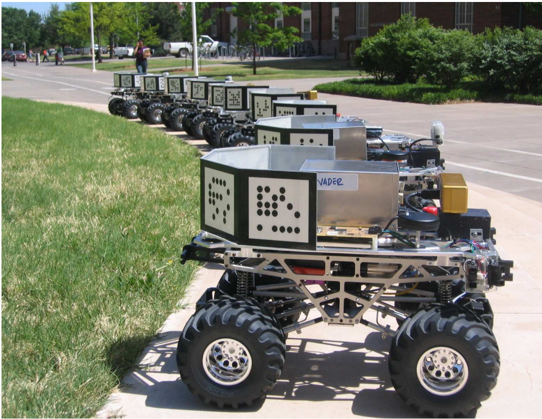
Figure 1: Multivehicle platform at Oklahoma State University. The platform consists of ten wirelessly networked robots based on the TXT-1 monster truck from Tamiya, Inc. Each robot is provided with a control board, odometry, various hot-swappable sensors, and an onboard embedded computer.
