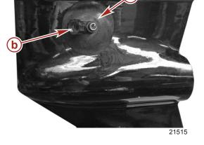
Flushing attachments for dual water pickup
