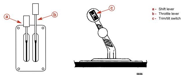
**Shift lever** - Shift functions are controlled by the movement of the shift lever. Shift into reverse by moving the shift lever to its aft position. Shift into neutral by moving the shift lever to its center position. Shift into forward by moving the shift lever to its forward position.
