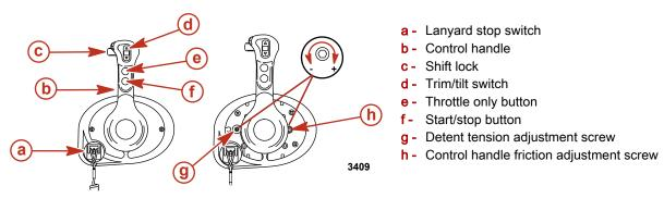
**Lanyard stop switch -** Turns the ignition off whenever the operator (when attached to the lanyard) moves far enough away from the operator's position to activate the switch. Refer to **Lanyard Stop Switch** for information on the use of this switch.
