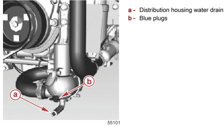
10. Check to ensure water drains out of the seawater pump housing.
