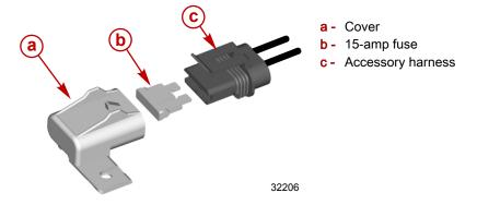
This power package uses a clean power harness that is connected to the engine starting battery. This clean power harness minimizes an excessive voltage drop to the engine and drive digital control electrical system. This harness is protected by a 5-amp fuse and is located near the engine starting battery.
