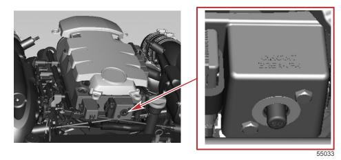
All of the engine protection fuses are located at the front of the engine. To access the fuses, disengage the fuse holders from the electrical plate assembly.
