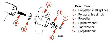
NOTE: The torque stated is a minimum torque value.
