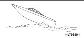
Operating recreational boats over waves and wakes is a natural part of boating. However, when this activity is done with enough speed to force the boat hull partially or completely out of the water, certain hazards arise, particularly when the boat reenters the water.
