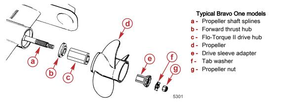
**NOTE:** The specified torque is a minimum torque value.
