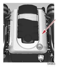
b. Lift up on the front of the second cover to disengage the cover from the front grommets. Pull the cover towards the front of the vessel to remove it from the two rear grommets
