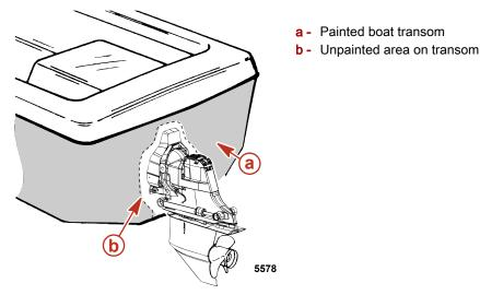
2. **Painting the sterndrive unit or transom assembly**: The sterndrive unit and transom assembly should be painted with a good-quality marine paint or an antifouling paint that does not contain copper, tin, or any other material that could conduct electrical current. Do not paint drain holes, anodes, MerCathode system, or items specified by the boat manufacturer.
