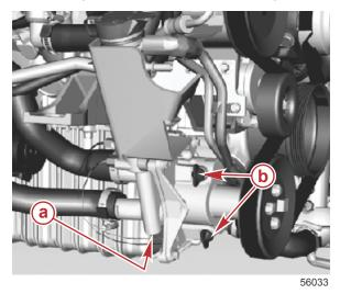
a - Seawater pump housing water drain **b** - Blue plugs
