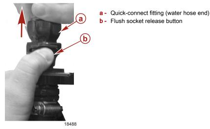
18. Remove the quick-connect fitting from the water hose.
