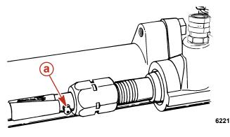
a - Steering cable grease fitting
