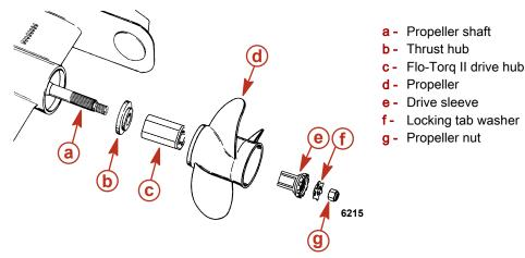
1. Apply a liberal coat of one of the following lubricants to the propeller shaft.
