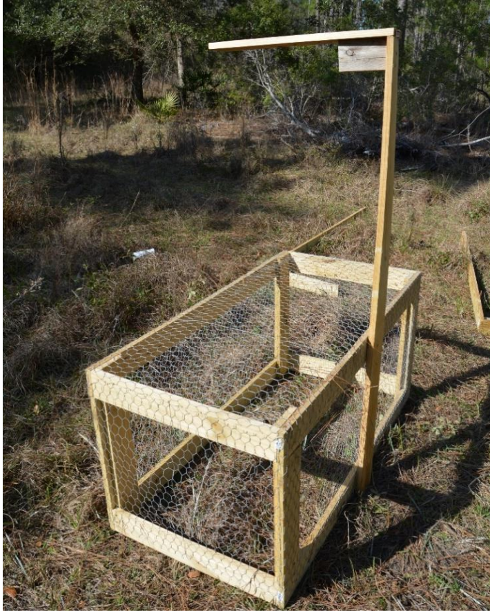
Figure B-9. Cage designed to inhibit scavenger activity and interference with specimens. Photo courtesy of Author.
