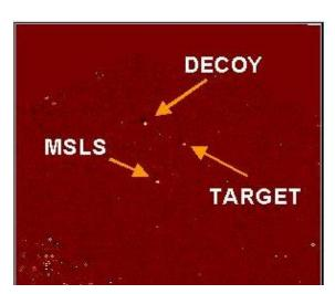
Until about two seconds before impact, the objects simply appear as points of light to the kill vehicle. The kill vehicle is able to recognize each object based on stored information it has about the objects' brightness and fluctuation. SOURCE: NANCE 2001
