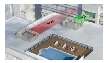
The low sound condenser fans paired with the radiated sound data of the unit operating at full load allows proper design with actual tested data. For example, if equipment is too loud or placed too closely to other buildings, corrective actions can be time consuming and costly. Greenheck provides low sound condenser fans as standard, offering an average sound power reduction of 5 to 8 decibels when compared to typical condenser fans.
