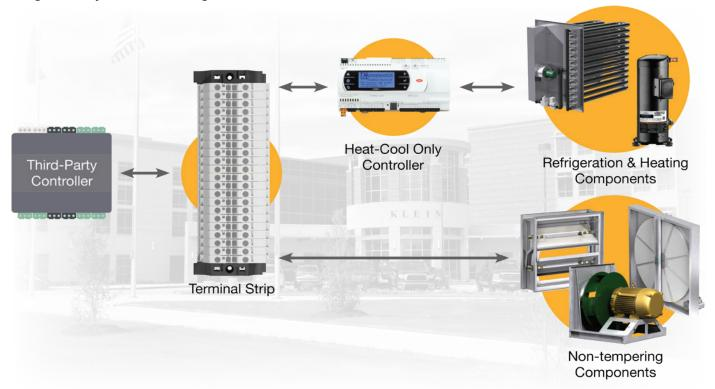
Listed below are the options available for a third-party to control and monitor through either digital or analog signals. The signals would need to be field wired from the third-party controller to the terminal strip provided in the RV/RVE/RVC unit.
