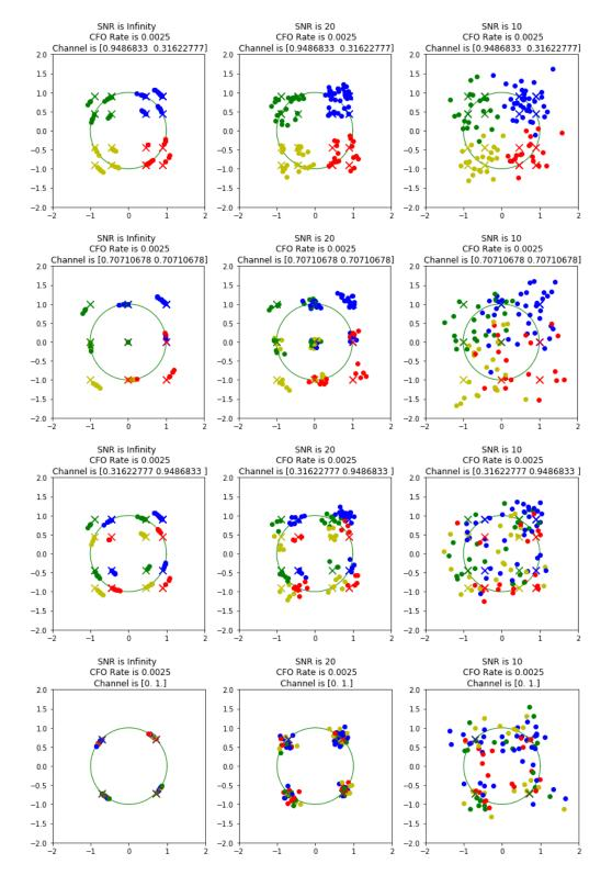
Figure 1.3: The effects of a two tap channel and a carrier frequency offset on the QPSK constellation.
