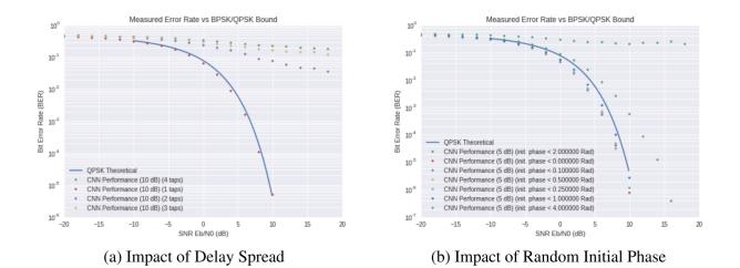
Figure 1.4: The impacts of multipath channels and initial phase offsets on bit error performance [17]. Note, the network is not re-trained for each new environment. As the number of paths and carrier frequency offset increase, the performance of the CNN decreases.
