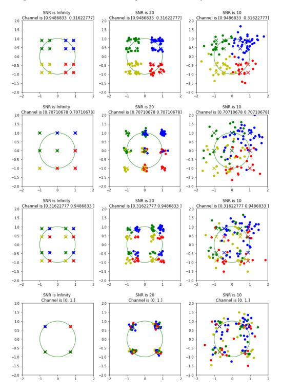
Figure 1.1: The effects of a two tap channel on the QPSK constellation.
