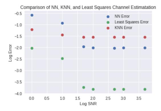
Figure 2.1: Comparison of a neural network, a K-Nearest-Neighbors, and a least-squares channel estimators for two tap, real channels.
