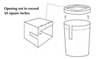
**Note:** This diagram is for illustration purposes only. Cubby boxes may be constructed of any material and openings may be restricted with wire mesh, wood strips or other material.
