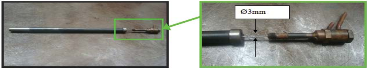
Fig. 6 Core pin cooling system.
