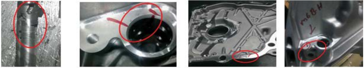
Fig. 4 Blow hole location on machined surface.
