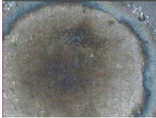
Figure B.24 SWS24B- Burnt Spot & Geometry
