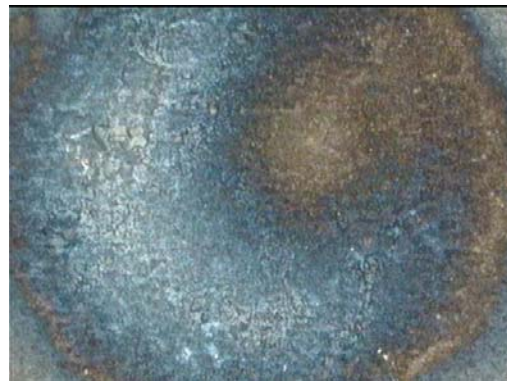
Figure B.62 SWS62B- Microcracks & Wide HAZ & Cu
