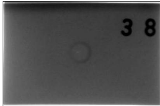
Figure C.38 SWS38- Burnt Spot (Small Hole)
