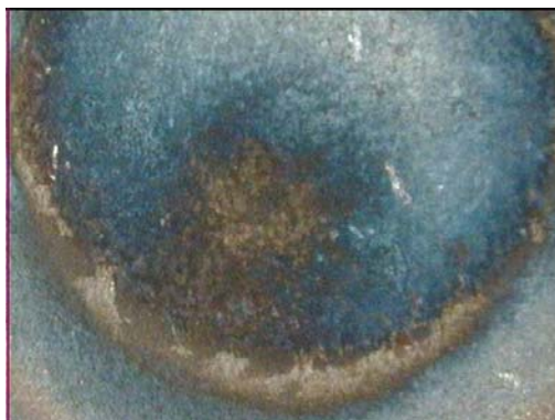
Figure B.45 SWS45B- Burnt HAZ
