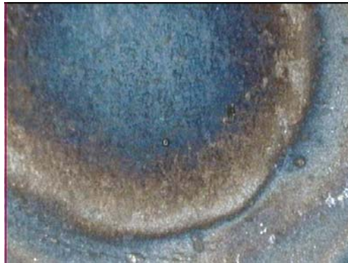
Figure B.20 SWS20B- Wide HAZ & Geometry
