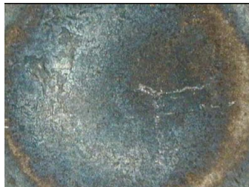
Figure B.58 SWS58B- Burnt Spot & Wide HAZ
