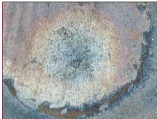
Figure B.22 SWS22B- Wide HAZ & Geometry & Cu
