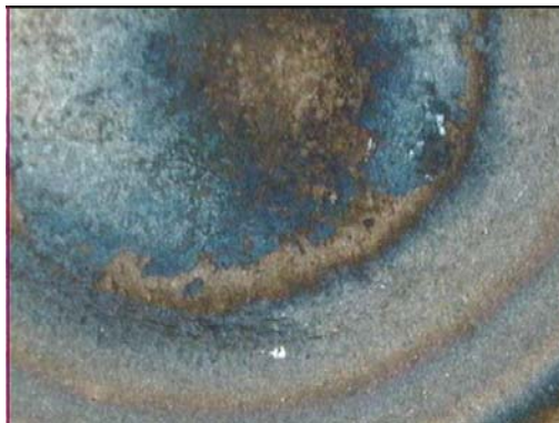
Figure B.21 SWS21B- Burnt Spot & Wide HAZ
