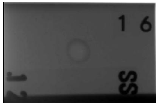
Figure C.16 SWS16- Burnt Spot & Wide HAZ
