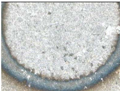
Figure B.75 SW75B- Pores & Narrow HAZ
