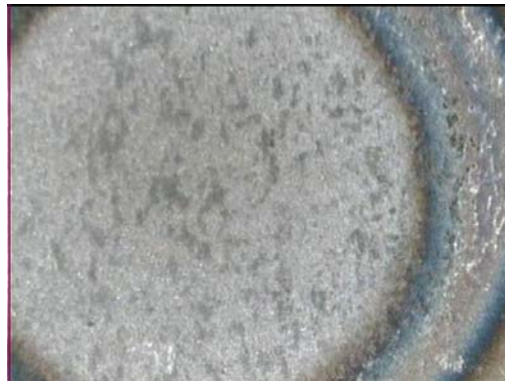
Figure B.32 SWS32F- Grains on Spot & HAZ
