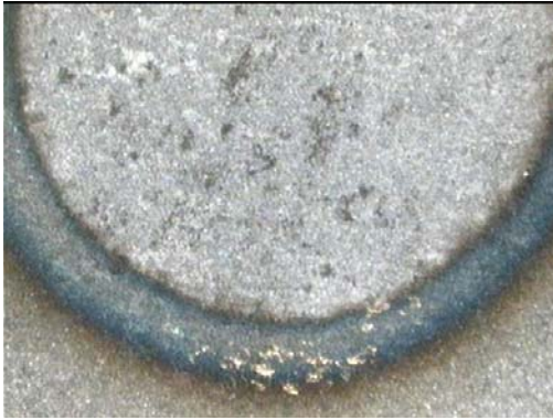
Figure B.59 SWS59B- Pores & Narrow HAZ
