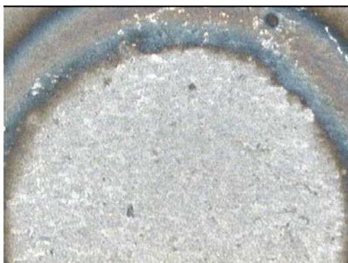
Figure B.69 SWS69B- Unsymmetric HAZ
