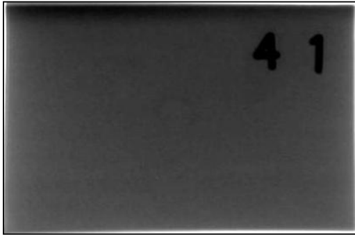
Figure C.39 SWS39- Gas Cavity
