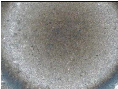
Figure B.61 SWS61F- Pores & Wide HAZ
