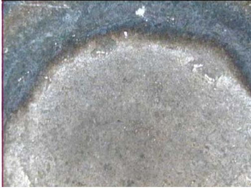
Figure B.11 SWS11B- Unsymmetry on HAZ
