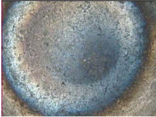
Figure B.5 SWS05B- Burnt and Copper pickup
