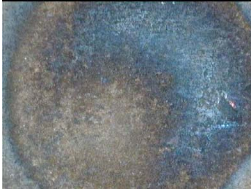
Figure B.65 SWS65B- Burnt Spot & Large HAZ
