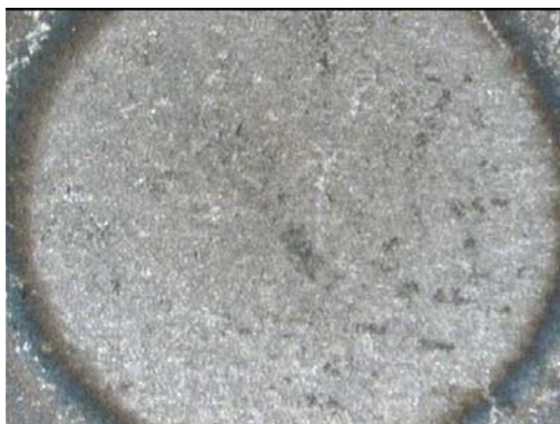
Figure B.87 SWS87F- Pores
