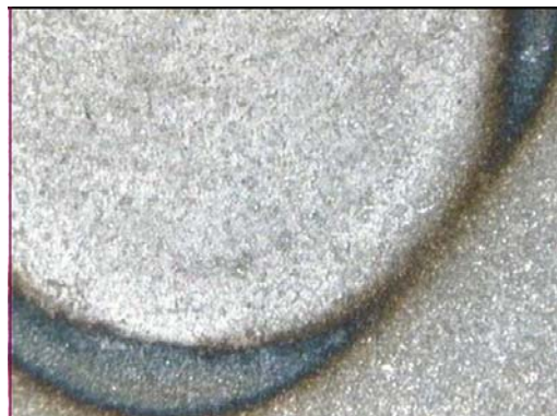
Figure B.8 SWS08B-Unsymmetry on the HAZ border
