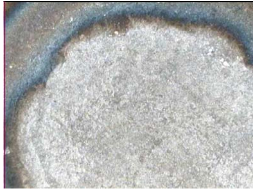
Figure B.8 SWS08B-Unsymmetry on the HAZ border
