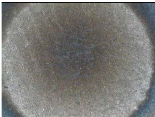
Figure B.99 SWS99F- Burnt Spot
