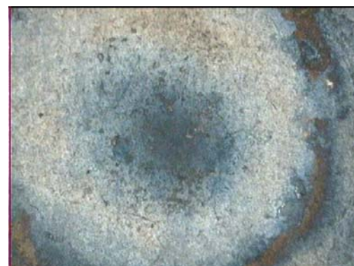
Figure B.16 SWS16B- Large HAZ & Burnt Spot
