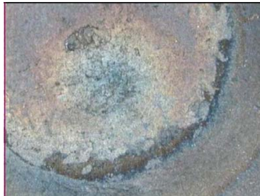
Figure B.26 SWS26B- Burnt Spot & Wide HAZ & Cu
