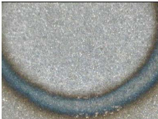
Figure B.55 SWS55F- Geometry & Narrow HAZ
