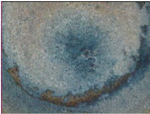
Figure B.49 SWS49B- Microcrack in Burnt Spot
