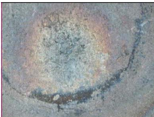
Figure B.27 SWS27B- Burnt Spot & Wide HAZ & Cu
