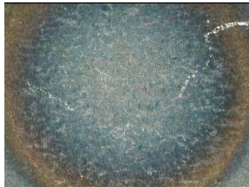
Figure B.98 SWS98F- Burnt Spot & Large HAZ
