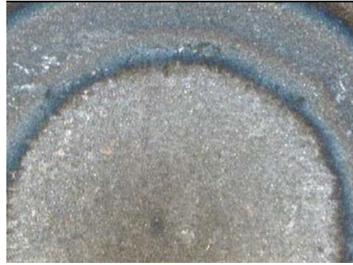
Figure B.90 SWS90B- Large HAZ
