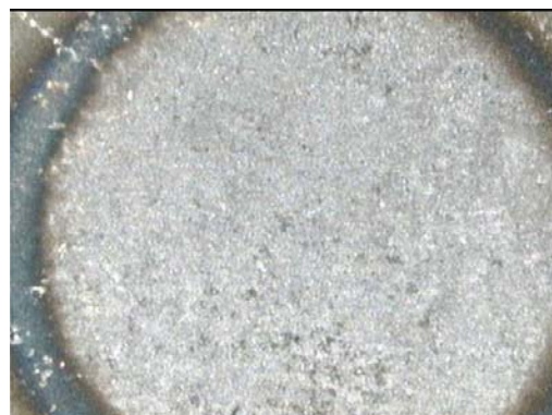
Figure B.70 SWS70F- Micropores
