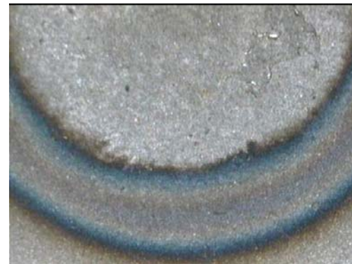
Figure B.54 SWS54F- Burnt Spot & Wide HAZ
