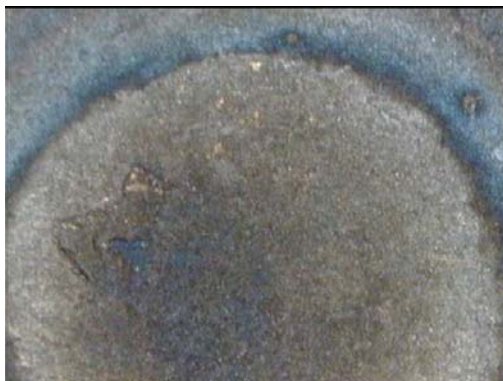
Figure B.55 SWS55F- Geometry & Narrow HAZ
