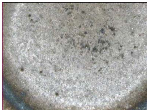
Figure B.4 SWS04F- Microholes on the spot
