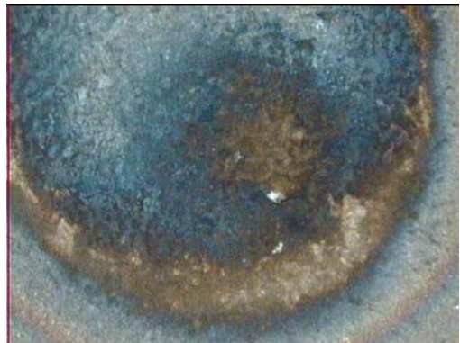
Figure B.38 SWS38B- Burnt HAZ
