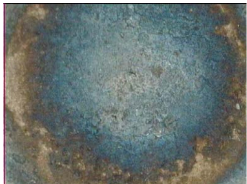
Figure B.40 SWS40B- Burnt & Spot&Wide HAZ
