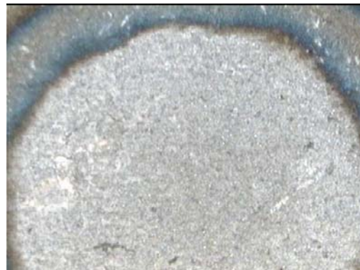
Figure B.68 SWS68B- Unsymmetric HAZ
