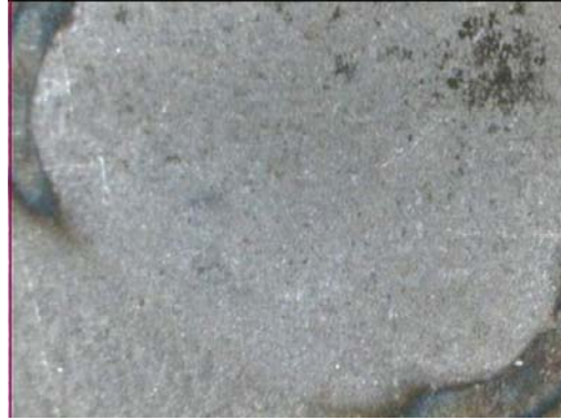
Figure B.12 SWS12B- No HAZ in LL portion
