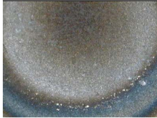
Figure B.54 SWS54F- Burnt Spot & Wide HAZ
