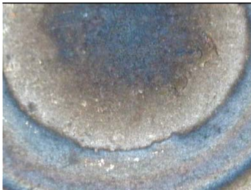
Figure B.67 SWS67B- Burnt Spot & Large HAZ
