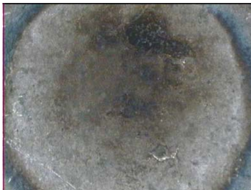
Figure B.39 SWS39B- Burnt Spot & Microcrack
