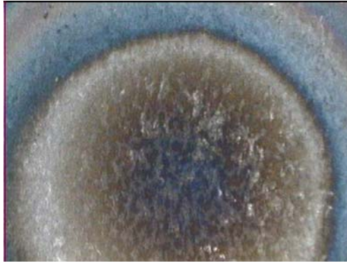
Figure B.35 SWS35F- Burnt Spot & Wide HAZ
