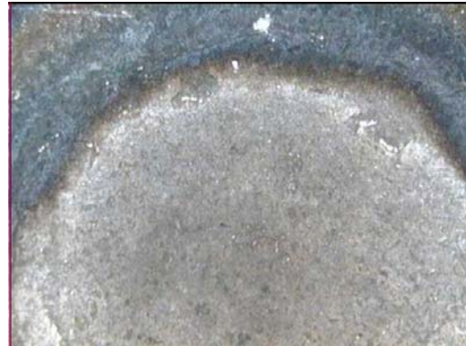
Figure B.84 SWS84B-Unsymmetry on HAZ Border
