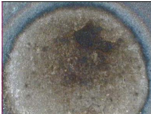
Figure B.37 SWS37B- Burnt Spot & Wide HAZ
