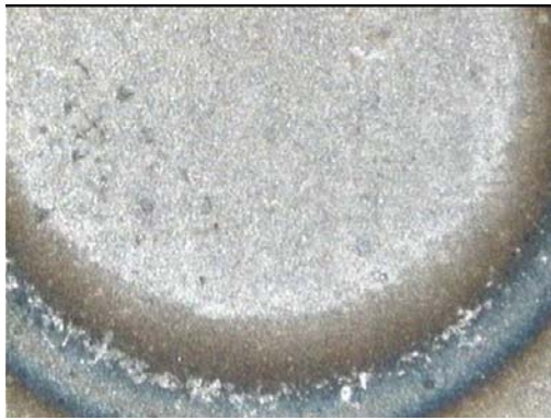
Figure B.95 SWS95F- Pores
