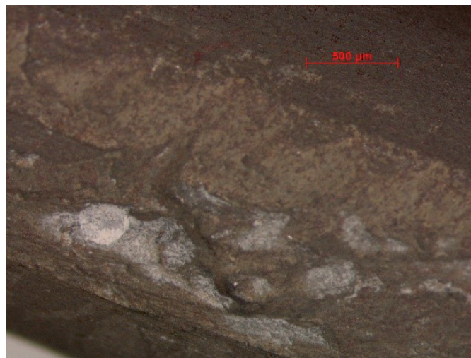
Fig. 1 – Slivers detected on the wire after the drawing
