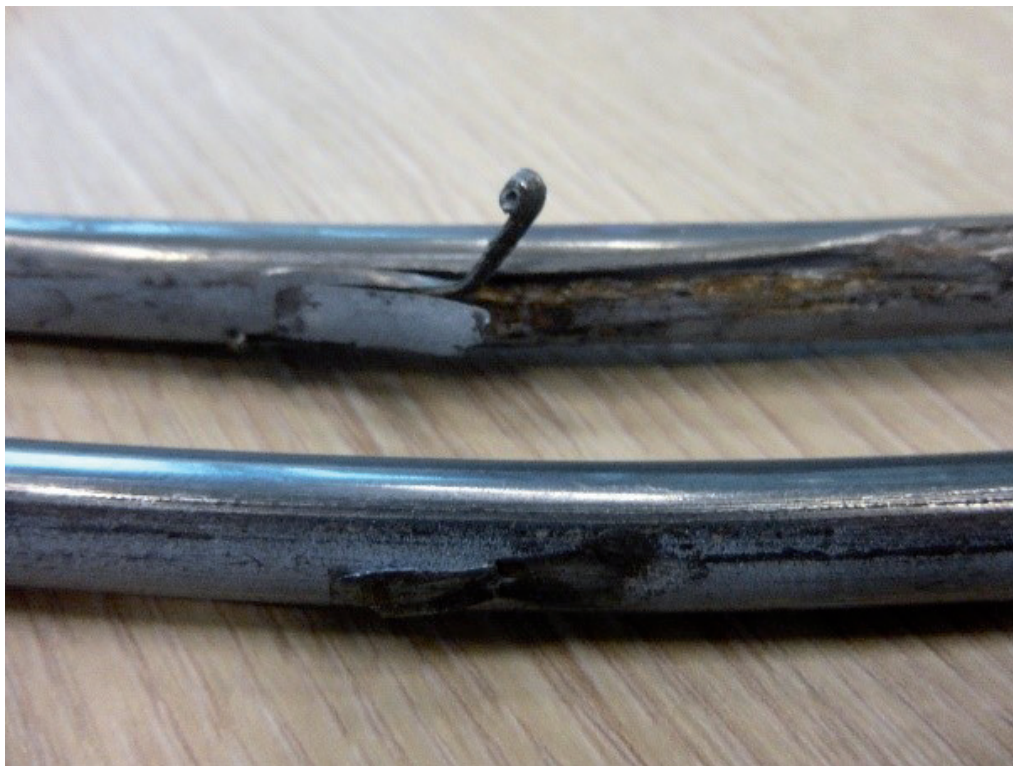
Fig. 3 – Laminations on wire drawn products (diameter 7mm).
