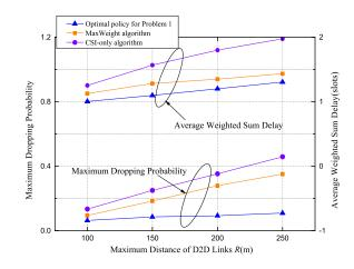
Fig. 5. The average weighted sum delay and the maximum dropping probability over all connections versus the maximum distance of D2D links R with  $\lambda = 1.5$  packets/slot and  $d_{max} = 0.1$ .
