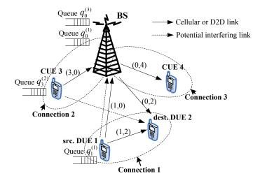
Fig. 1. A simple OFDMA cellular network with D2D communications.
