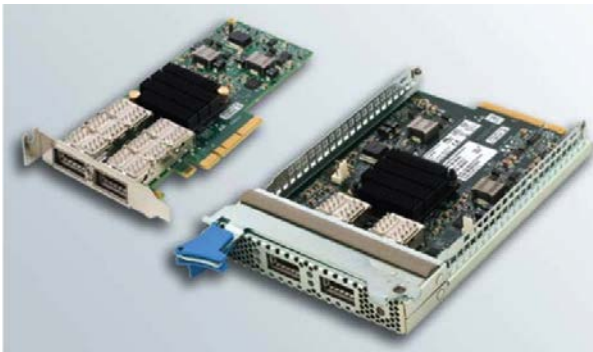
Figure 20. Sun Dual Port 4x IB QDR Host Channel Adapter PCIe M2 and Sun Dual Port 4x IB QDR Host Channel Adapter ExpressModule M2.
