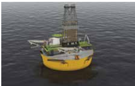
◆ The SSP Driller is customisable for mid to ultra-deepwater drilling and is capable of increased variable deck load over existing technologies
