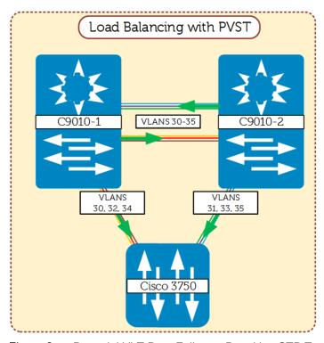
Figure 3 Potential VLT Peer Failure – Resulting STP Topology
