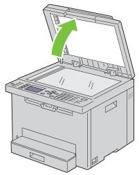
2 Place the document face down on the document glass and align it with the registration guide on the top left corner of the glass.
