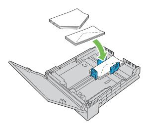
To prevent DL and Monarch from being wrinkled, they are recommended to be loaded with the flaps opened. Place the print side facing up, and the flaps come at the bottom when you face towards the printer.
