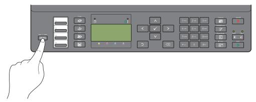
2 Start the WPS operation on the wireless LAN access point (Registrar) or router within 2 minutes. When the wireless LAN connection setting is completed, the **WiFi** (Wi-Fi | WPS) button lights up.
