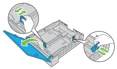
**NOTE:** When loading legal size or user-specified print media, slide the extendable part of the tray while pinching the lever.
