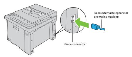
If the phone communication is serial in your country (such as Germany, Sweden, Denmark, Austria, Belgium, Italy, France and Switzerland), and you are supplied with a yellow terminator, insert the yellow terminator into the phone connector ( C.).
