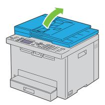
**8** Remove the document from the ADF feed roller or the feed area by carefully pulling the document in the direction of the arrow shown in the following illustration.
