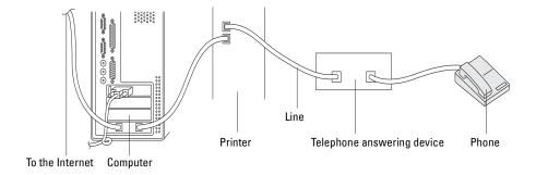
If you want to use your computer modem for faxing or for a dial-up Internet connection, connect the computer modem directly to the back of your printer with the TAD as shown above.
