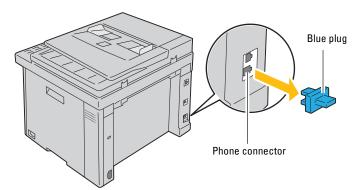
**3** To connect a telephone and/or answering machine to your printer, plug the telephone or answering machine line cord into the phone connector ( ).
