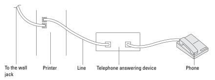
You can connect a telephone answering device (TAD) directly to the back of your printer as shown above.
