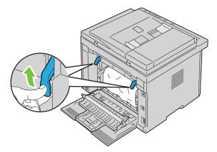
Remove any jammed paper from the back of the printer.
