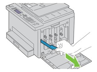
6 Insert the cleaning rod fully into the hole beside the arrow on the printer until its tip reaches the interior of the printer as illustrated below, and then pull it out.
