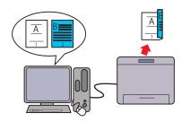
Manual Duplex Print feature allows you to print two or more pages on the front and back side of a single sheet of paper manually. Using this feature, you may reduce the paper consumption.
