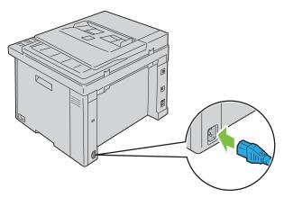
**2** Connect the other end of the cable to the power source.
