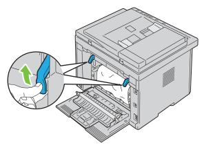
3 Remove any jammed paper from the back of the printer. If no paper is found in the paper path, face the front of the printer and check the output tray.
