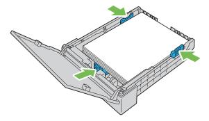
**6** After confirming that the guides are adjusted and secured, close the dust cover and insert the tray into the printer. Inserting back the tray displays the message on the LCD panel prompting you to specify the paper size in the tray.
