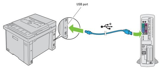
**3** Connect the other end of the cable into a USB port of your computer.
