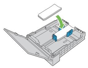
CAUTION: Never use envelopes with windows, or coated linings. These lead to paper jams and can cause damage to the
