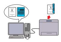
Manual Duplex Print feature allows you to print two or more pages on the front and back side of a single sheet of paper manually. Using this feature, you may reduce the paper consumption.
