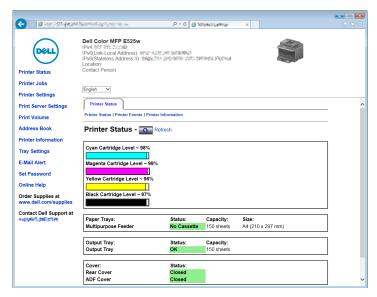
To fill out printer inventory reports requiring the asset tag number of all the printers in your area, use the **Printer Information** feature in the **Dell Printer Configuration Web Tool**. Enter the IP address of each printer on the network to display the asset tag number.
