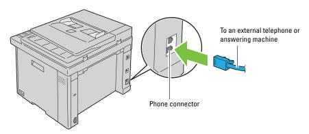
If the phone communication is serial in your country (such as Germany, Sweden, Denmark, Austria, Belgium, Italy, France and Switzerland), and you are supplied with a yellow terminator, insert the yellow terminator into the phone connector ( ).
