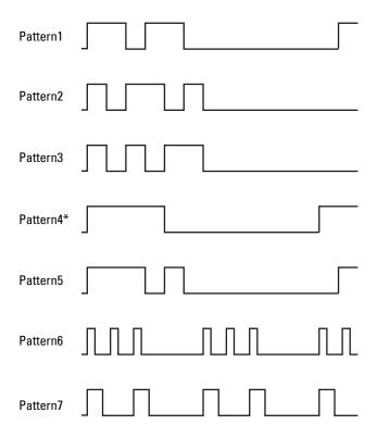
Ask your telephone company which pattern you need to select to use this service. For example, Pattern 7 is the New Zealand FaxAbility distinctive ringing pattern: rings for 400ms, stops for 800ms, rings for 400ms and stops for 1400ms. This pattern is repeated over and over again. This printer only responds to Distinctive Alert cadence(s) DA4 in New Zealand.
