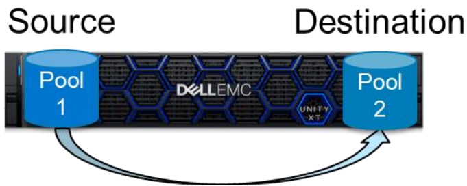
Figure 32 Local asynchronous replication
