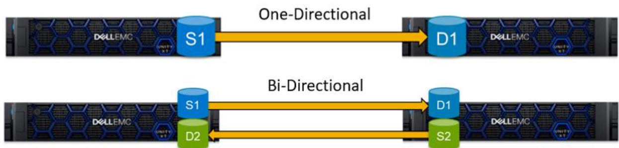
Figure 3 Supported synchronous block replication topologies
