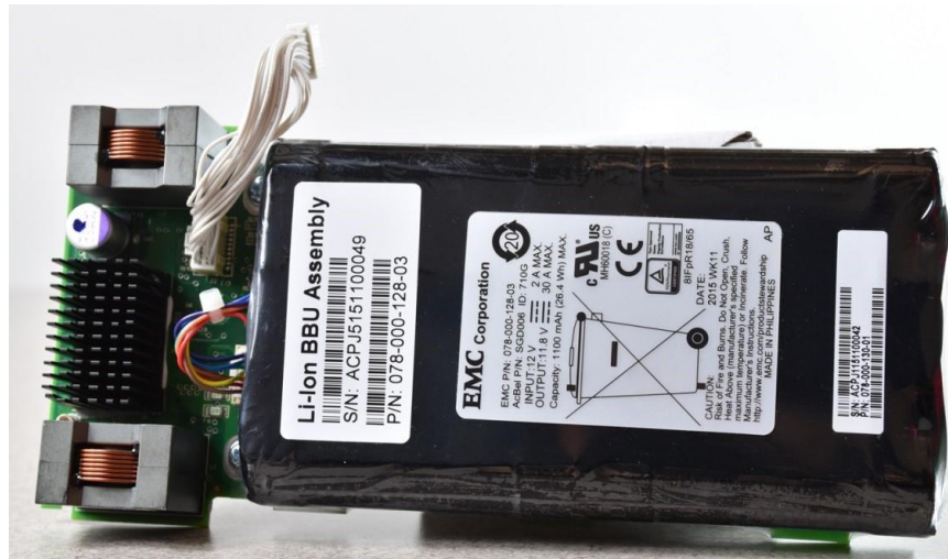
Figure 6. Battery Backup Unit (380/F)
