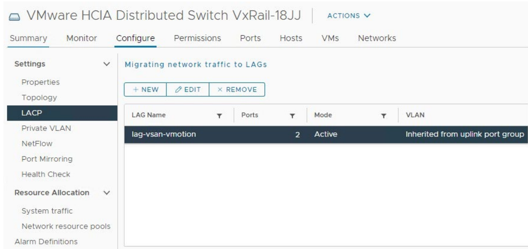
Figure 50. Sample LACP policy configured on virtual-distributed- switch.
