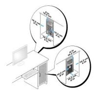
If your computer is installed in a corner on a desk or under a desk, leave at least 5.1 cm (2 in) clearance from the back of the computer to the wall to permit the airflow required for proper ventilation.
