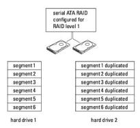
If a drive failure occurs, subsequent read and write operations are directed to the surviving drive. A replacement drive can then be rebuilt using the data from the surviving drive. Also, because data is duplicated on both drives, for example, two 120-GB RAID level 1 drives collectively have a maximum of 120-GB on which to store data.
