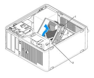
NOTICE: Unless a new heat sink is required for the new processor, reuse the original heat sink assembly when you replace the processor.
