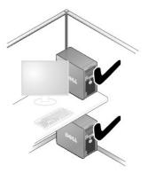
NOTICE: Do not install your computer in an enclosure that does not allow airflow. Restricting the airflow impacts your computer's performance, possibly causing it to overheat.
