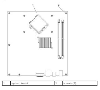
9. Place the system board that you just removed next to the replacement system board to compare and ensure they are identical.
