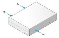
5. Align the shoulder screws on the optical drive with the shoulder screw slots, and slide the drive into the bay until it clicks into place.
