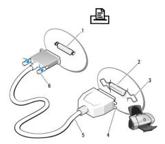
1 parallel connector on computer 2 connector on printer
