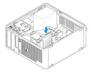
6. Connect the power and data cables to the drive.
