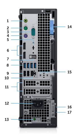
1 Line-out audio port 2 PS2 Port (Keyboard) 3 4 Serial port PS2 Port (Mouse) 5 DisplayPort/HDMI 2.0b/VGA/USB Type-C Alt-Mode (optional) 6 DisplayPorts (2) 7 8 USB 3.1 Gen 1 ports (4) Service tag label 9 USB 2.0 ports (2) (one supports, SmartPower On) 10 Network port 12 11 Expansion card slots Power connector port 13 14 Power supply diagnostic light Release latch 15 External SMA antenna connectors (optional) 16 Kensington security cable slot 17 Padlock ring
