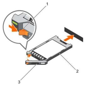
Figure 97. Installing a 1.8 inch hot-swappable uSATA SSD carrier
