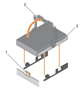
Figure 27. Removing a hard drive carrier from the hard drive tray
