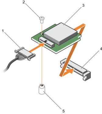
Figure 121. Installing the vFlash media unit
