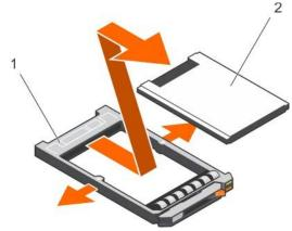
Figure 102. Removing a 1.8-inch hard drive into a hard drive carrier
