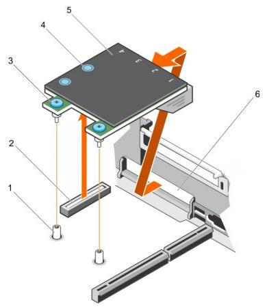
Figure 69. Removing the NDC
