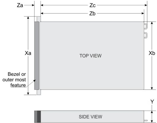
Figure 13. Chassis dimensions of the PowerEdge R730xd system
