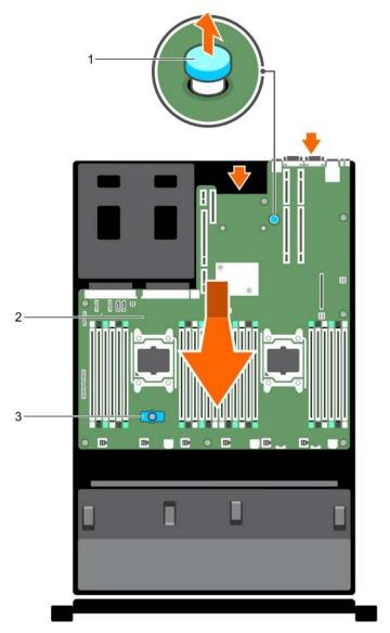
Figure 85. Removing the system board
