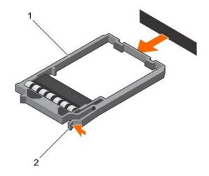
Figure 100. Removing a 1.8-inch hard drive blank
