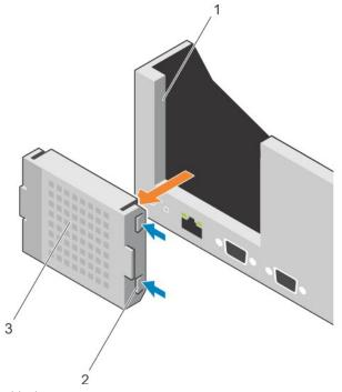
Figure 56. Removing the riser 1 blank
