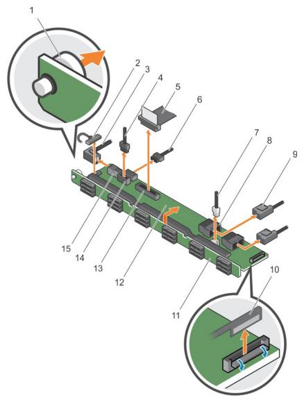
Figure 111. Removing the 1.8 Inch (x18) SAS/SATA backplane
