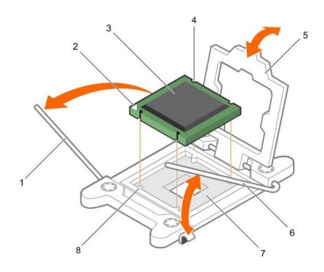
Figure 41. Removing and installing a processor
