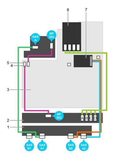
Figure 107. Cabling diagram—2.5 Inch (x24) SAS/SATA backplane (option 3)
