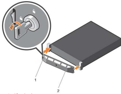
Figure 16. Installing the optional front bezel
