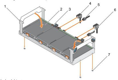
Figure 24. Installing the hard drive tray
