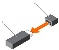
Figure 71. Removing the internal USB memory key
