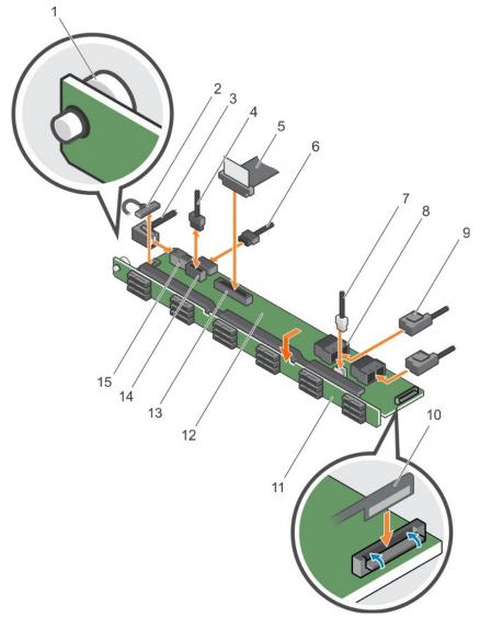
Figure 115. Installing the 1.8 Inch (x18) SAS/SATA backplane
