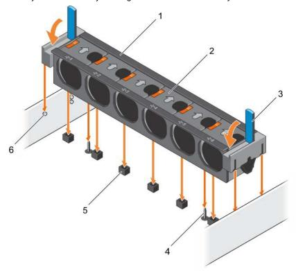
Figure 35. Installing the cooling fan assembly
