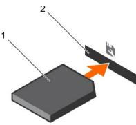
Figure 119. Installing the SD vFlash media card
