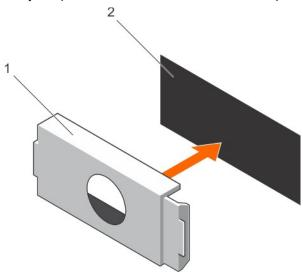
Figure 76. Installing the PSU blank
