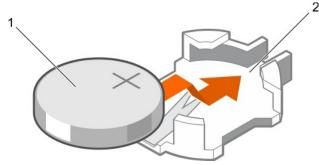
Figure 74. Installing the system battery
