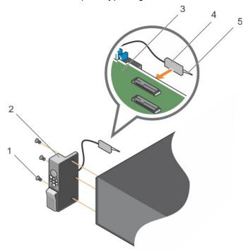
Figure 123. Installing the control panel
