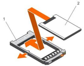
Figure 103. Installing a 1.8-inch hard drive into a hard drive carrier
