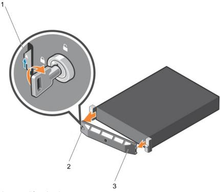
Figure 14. Removing the optional front bezel
