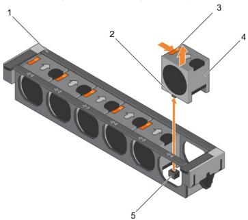
Figure 32. Removing a cooling fan
