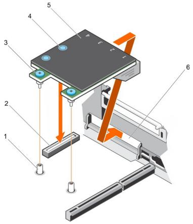
Figure 70. Installing the NDC
