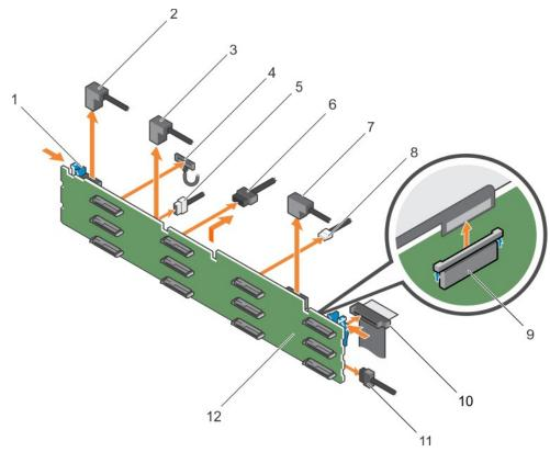
Figure 108. Removing the 3.5 inch (x12) SAS/SATA backplane
