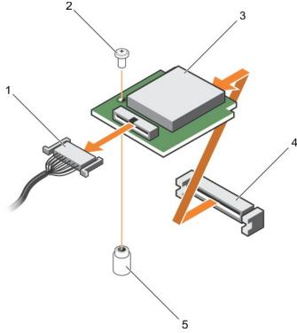
Figure 120. Removing the vFlash media unit
