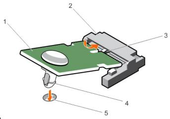
Figure 87. Installing the TPM
