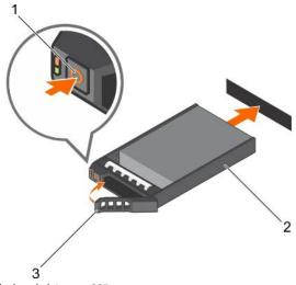
Figure 96. Installing a hot-swappable hard drive or SSD
