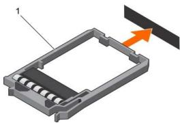
Figure 101. Installing a 1.8-inch hard drive blank
