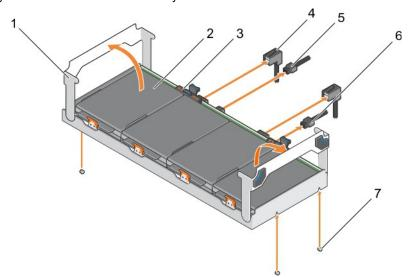
Figure 23. Removing the hard drive tray
