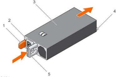
Figure 78. Installing an AC PSU
