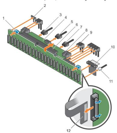
Figure 104. Removing the 2.5 inch (x24) SAS/SATA backplane
