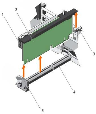
Figure 60. Removing the expansion card riser 2
