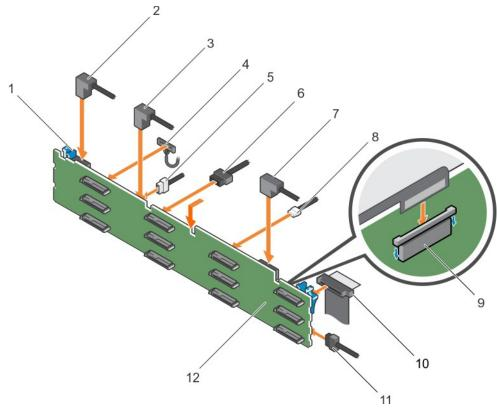
Figure 114. Installing the 3.5 inch (x12) SAS/SATA backplane
