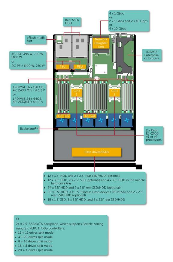
Figure 1. Supported configurations for the PowerEdge R730xd system
