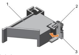
Figure 47. Closing the PCIe card holder latch
