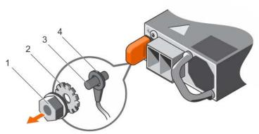
Figure 80. Removing the safety ground wire
