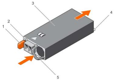
Figure 84. Installing a DC PSU
