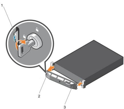
Figure 15. Removing the optional Quick Sync front bezel
