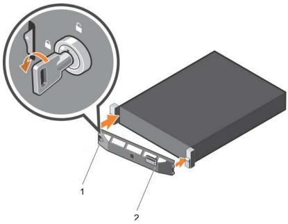
Figure 17. Installing the Quick Sync bezel
