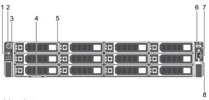
Figure 3.  $12 \times 3.5$ -inch hard drive chassis
