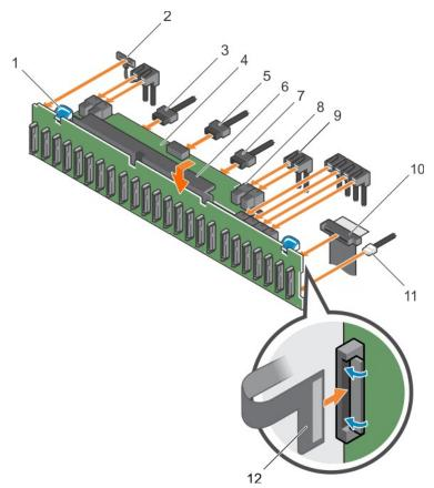
Figure 113. Installing the 2.5 inch (x24) SAS/SATA backplane
