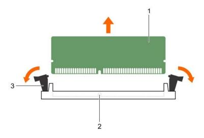
Figure 37. Removing the memory module
