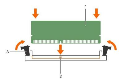
Figure 38. Installing the memory module
