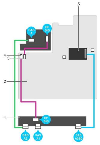
Figure 109. Cabling diagram—3.5 inch (x12) SAS/SATA backplane (option 1)
