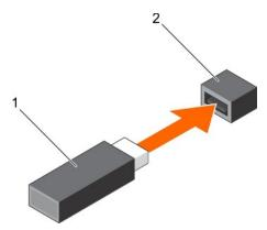
Figure 72. Installing the internal USB memory key
