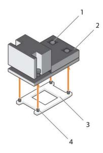
Figure 39. Removing a heat sink
