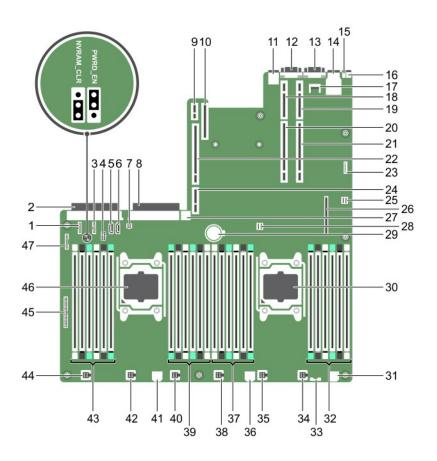
Figure 126. System board jumpers and connectors
