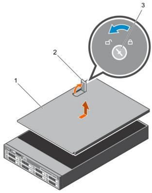
Figure 18. Removing the system cover
