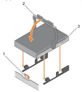
Figure 28. Installing a hard drive carrier into the hard drive tray
