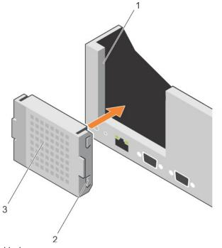
Figure 57. Installing the riser 1 blank
