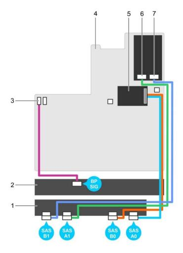
Figure 106. Cabling diagram—2.5 Inch (x24) SAS/SATA backplane (option 2)
