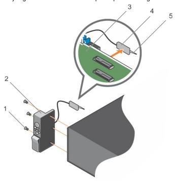
Figure 122. Removing the control panel
