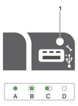
Figure 11. iDRAC Direct LED indicator
