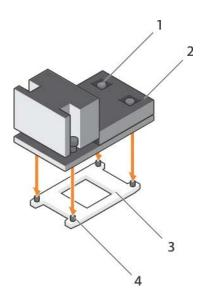
Figure 43. Installing the heat sink
