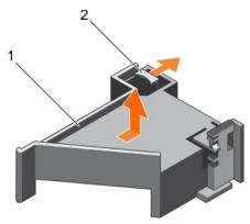
Figure 44. Removing the PCIe card holder
