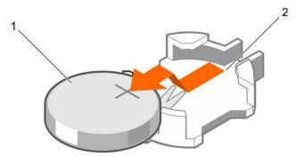
Figure 73. Removing the system battery
