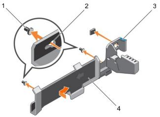
Figure 49. Installing the cable retention bracket
