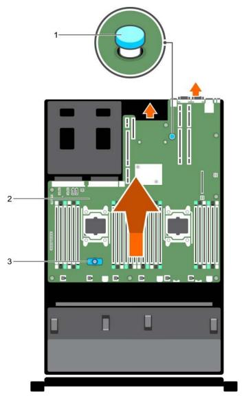
Figure 86. Installing the system board
