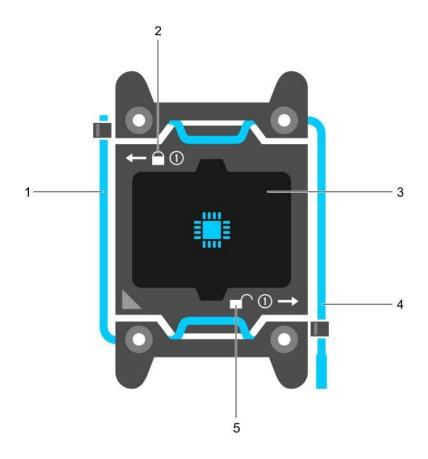
Figure 40. Processor shield
