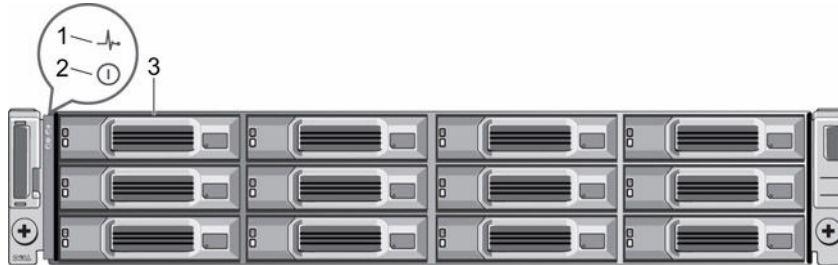
Figure 16. SC100 Front-Panel Features and Indicators
